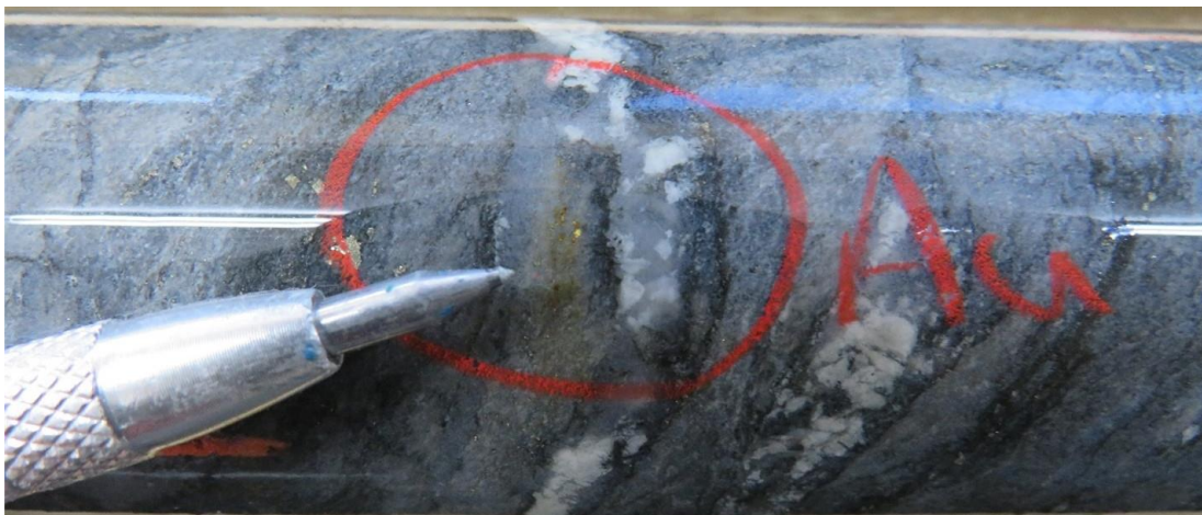
Figure 7.12 – Gold grain in a quartz-tourmaline vein selvage (ELM20-051 at a depth of 201.14 m)
