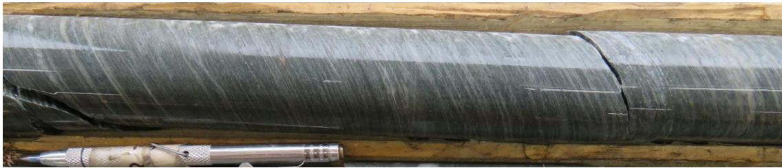
Figure 7.4 – Laminated ash tuff from drill hole ELM20-040 at a depth of 53 m
