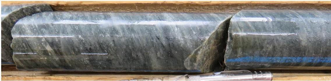
Figure 7.5 – Lapilli tuff from drill hole ELM20-040 at a depth of 77 m
