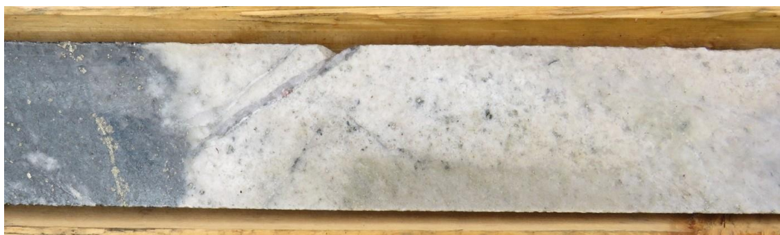
Figure 7.9 – Felsic intrusive from drill hole ELM20-010 at a depth of 168.8 m
