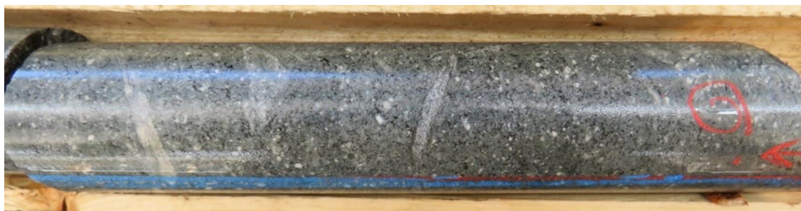
Figure 7.3 – Crystal and lapilli tuff from drill hole ELM21-019 at a depth of 109 m
