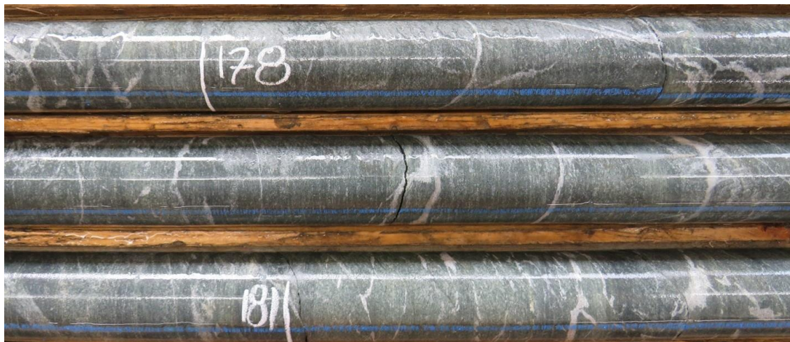
Figure 7.8 – Typical basalt injected by numerous calcite veinlets
