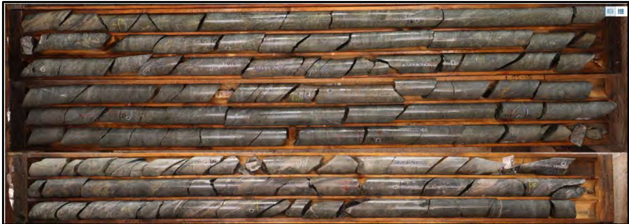
Figure 7.29 Core from IL-11-02 at Iris showing an interval of 8.39 g/t Au over 11.0 m focused on two quartz-carbonate-pyrite shear zones in a wider interval of silica-carbonate-altered andesite.
