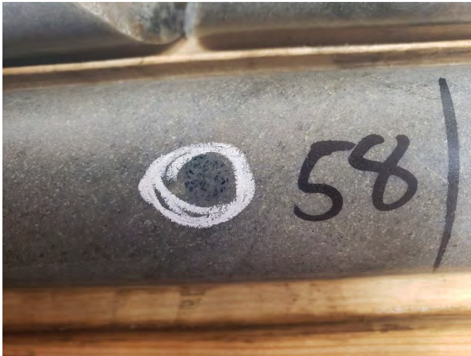
Figure 7.13. Results of Potassium Ferricyanide Stain-Testing for Iron Carbonates, Revealing Iron Carbonate Within a Zone of Silica-Carbonate-Altered Dacites, ML-03-009.
