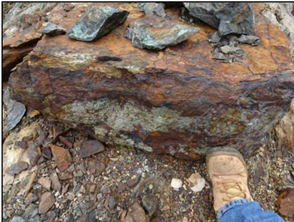
Figure 7.26. Gossanized chalcopyrite-magnetite mass in mineralized shear, main Hamlin stripped area.
