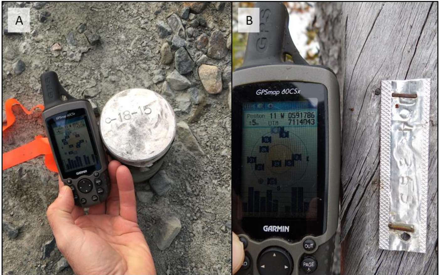
Figure 12-2: Examples of On-Site Collar Location Verifications
