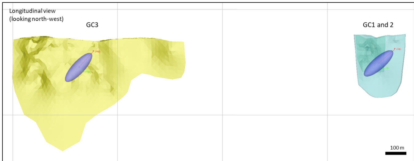
Figure 14-19: Longitudinal View of the Zone Wireframes and Search Ellipsoids (Pass 2) for the Goldcrest Deposit
