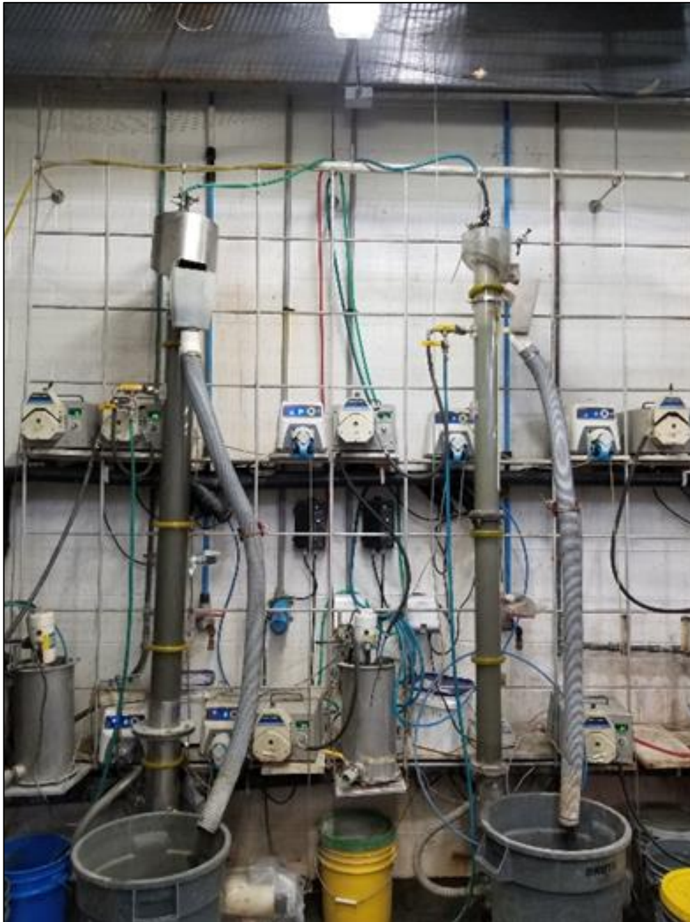
Figure 13-22: Eriez Pilot Plant 4" Diameter Rougher Column and 3" dia Scavenger Column
