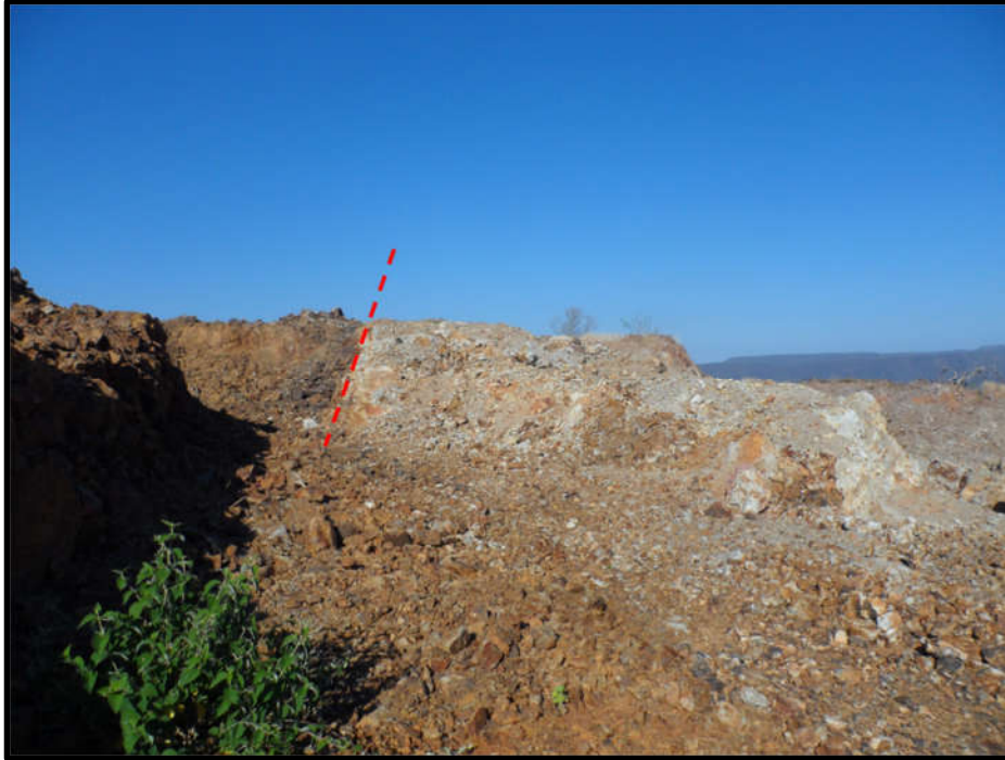
Figure 7-23: Nicho Norte Test Pit Showing Sub-Vertical Contact Between Andesite Tarahumara Formation (left) and Aplitic Porphyry QFP (right)
