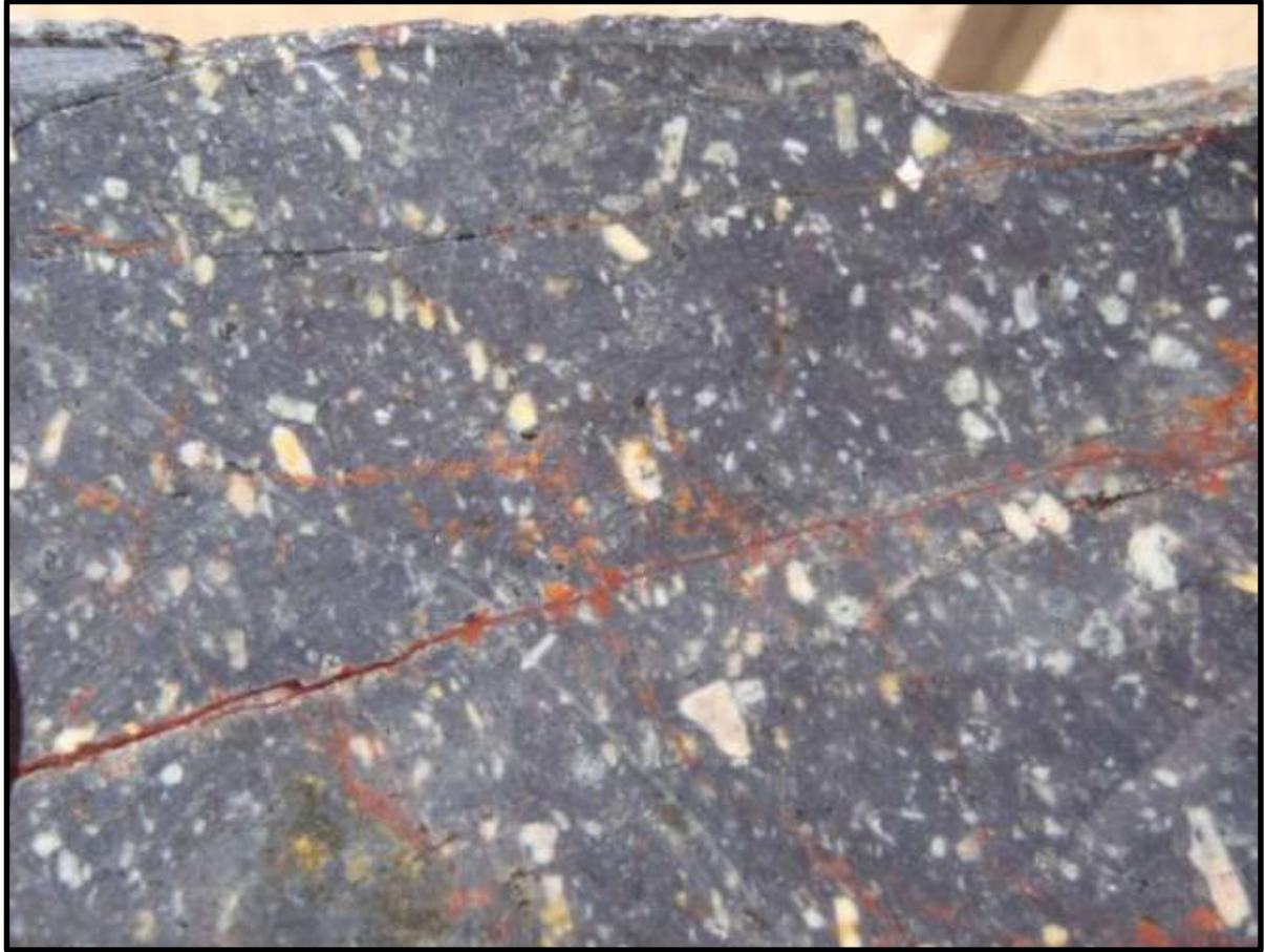
Figure 7-10: V12 Porphyritic Dacite Flow (Flow Texture is Not Apparent in this Rock Unit, S10-43D at 201 m)
