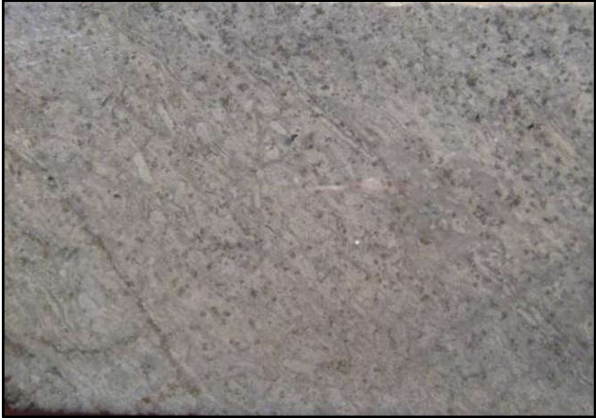
Figure 7-12: V14 Dacite Flow with Strong Sericitization of Feldspars and Silicification Along Flow Banding. Abundant Pyrite Disseminated and in Veinlets (S10–43D at 161 m).
