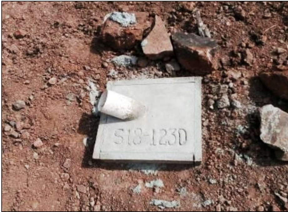
Figure 10-5: Typical Collar Completion at the Project
