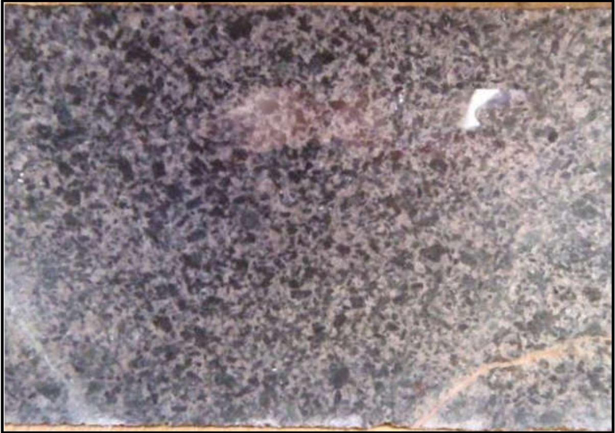
Figure 7-4: Fresh Monzonite (S10-063D). Plagioclase Phenocrysts Are of Dark-Grey Colour with a Reddish Matrix. Hornblende is Partially Altered to Chlorite.
