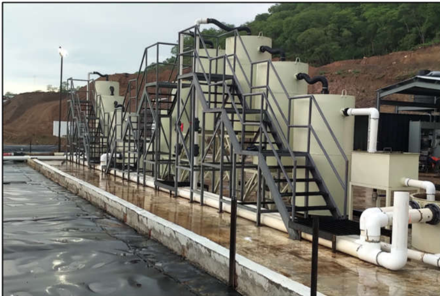
Figure 18-4: Gold Recovery (Carbon) Plant
