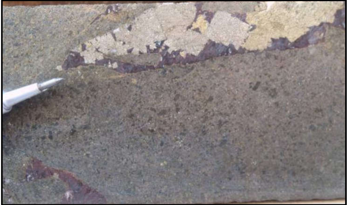
Figure 7-9: Nicho Area Chloritized Andesite with Hydrothermal Brecciation. Breccia Cemented with Dark Specular Hematite, Whitish Euhedral Pyrite, and Yellow Chalcopyrite.
