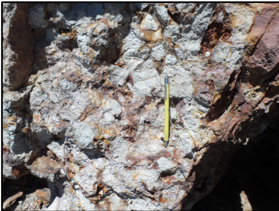
Figure 7-24: Nicho Norte Breccia Showing Fragments of Aplitic Feldspar Porphyry (QFP) Cemented by Quartz Calcite Veins
