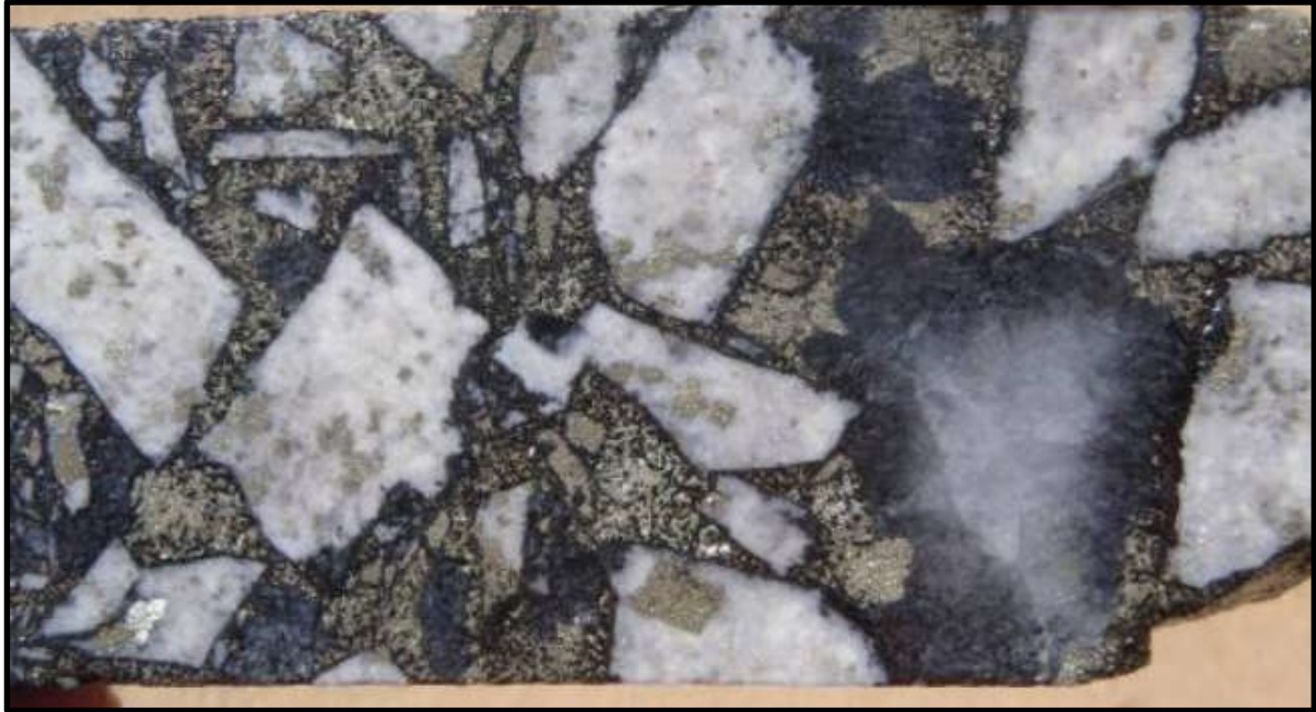
Figure 7-13: Quartz–Tourmaline–Pyrite Breccia with Clasts of Sericitized Monzodiorite Cemented by Sulphides and Minor Tourmaline (S11–122D at 275 m)
