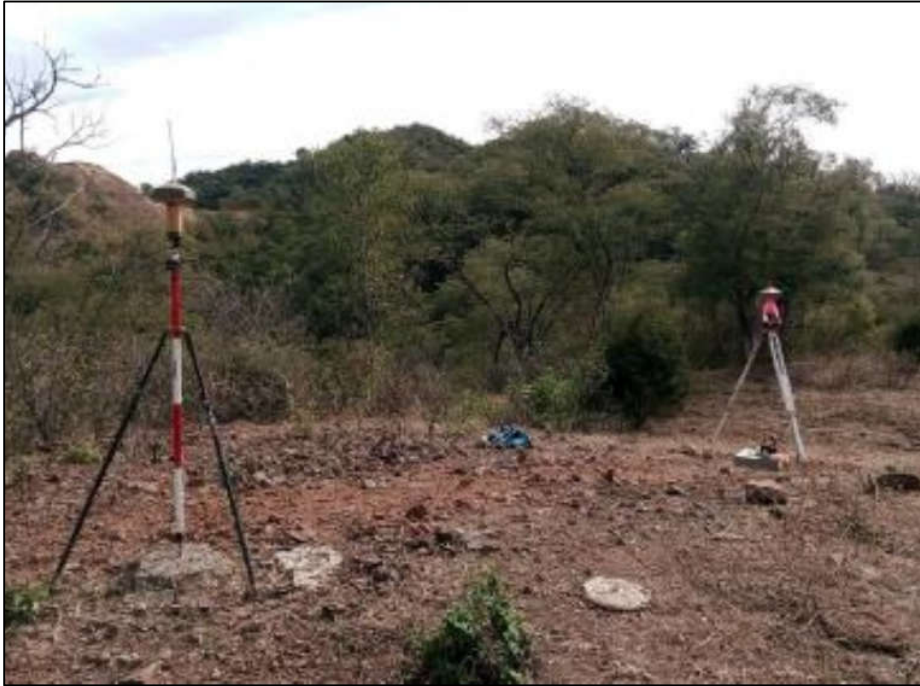
Figure 10-7: Surveying Site Control Points
