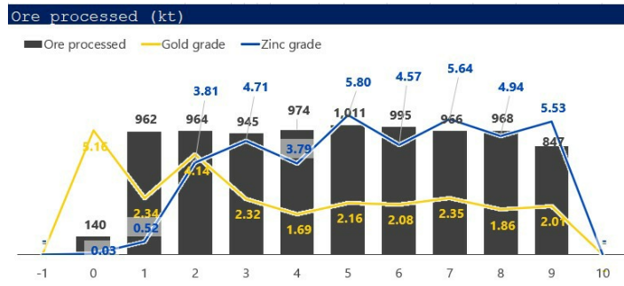
Figure 19-1: Materialized Material Processed and Grade Profiles for Gold and Zinc
