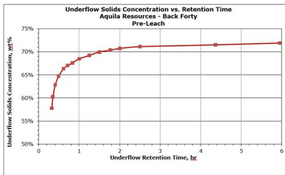
Figure 10-15: Underflow Solids Concentration Versus Retention Time – Aquila Resources – Back Forty
