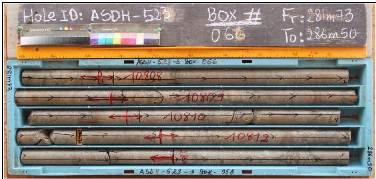
Figure 10-6: Diamond core photograph example
