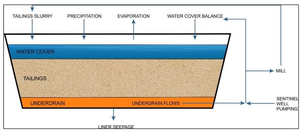
Figure 18-8: Inputs and Outputs for TMF Water Balance
