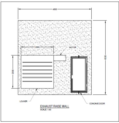
Figure 16-38: Exhaust Raise Bulkhead - Typical
