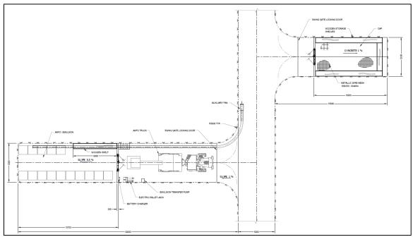
Figure 16-32: Explosive and Detonator Magazine Plan View
