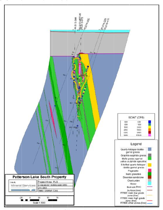
Figure 13-2: Location of Metallurgical Drill Holes - Section S330E
