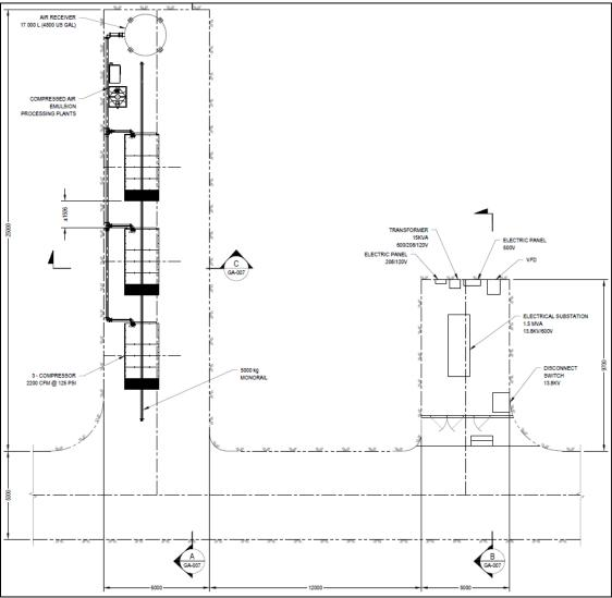
Figure 16-39: 400 Level Compressor and Electrical Room
