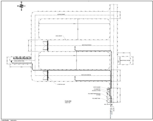
Figure 16-31: Sump Decantation Station Arrangement
