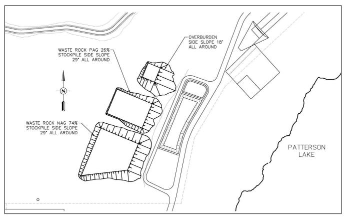
Figure 18-3: General Arrangement of Waste Rock and Mine Backfill Material Storage Stockpiles
