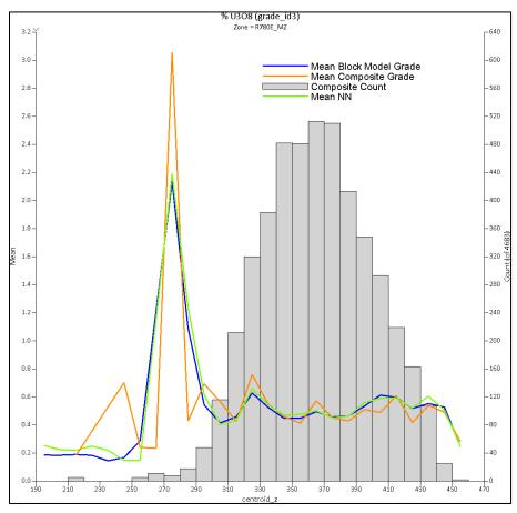
Figure 14-22: Vertical (Z) Swath Plot of R780E\_MZ Deposit
