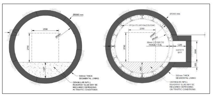
Figure 16-5: Decline Tunnel Cross Section
