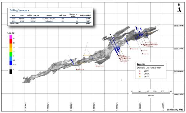
Figure 10-3: R780E Exploration Infill Drill Hole Location Map Completed 2019–2021
