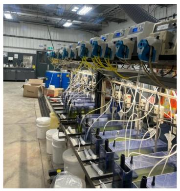
Figure 13-5: Continuous SX Mini Pilot Test Set-Up
