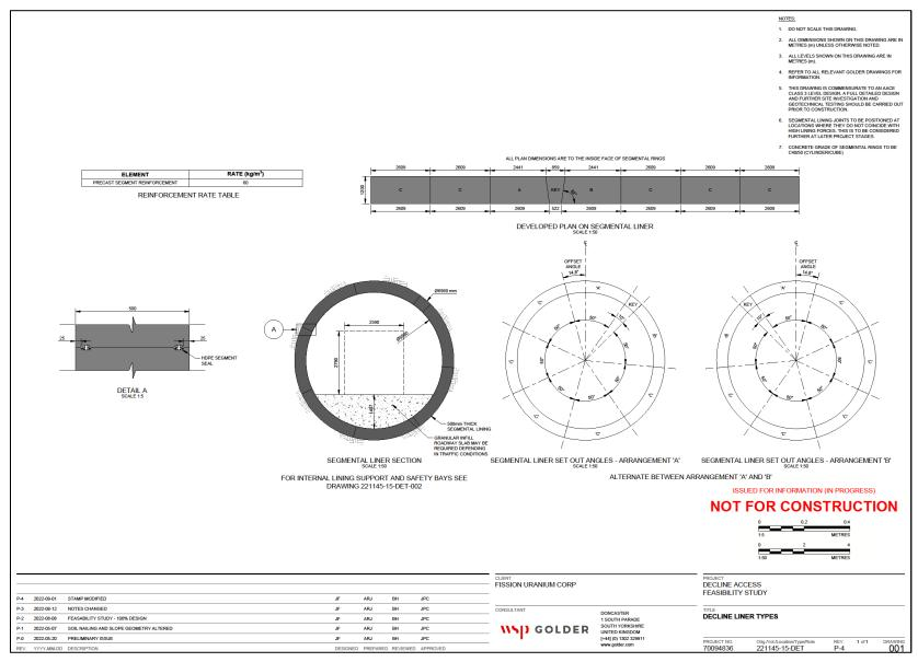
Figure 16-4: Decline Liner Section and Concrete Segment Arrangement
