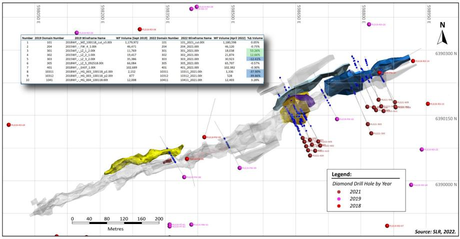
Figure 14-5: 2022 R780E LG and HG Wireframe Volume
