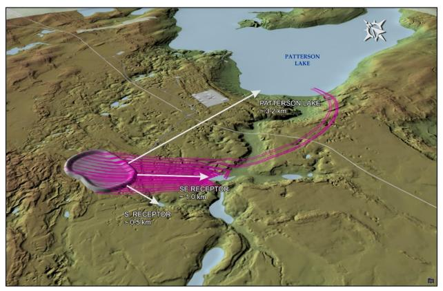
Figure 18-11: Particle Tracking Analysis Showing Solute Migration Pathways to Potential Receptors
