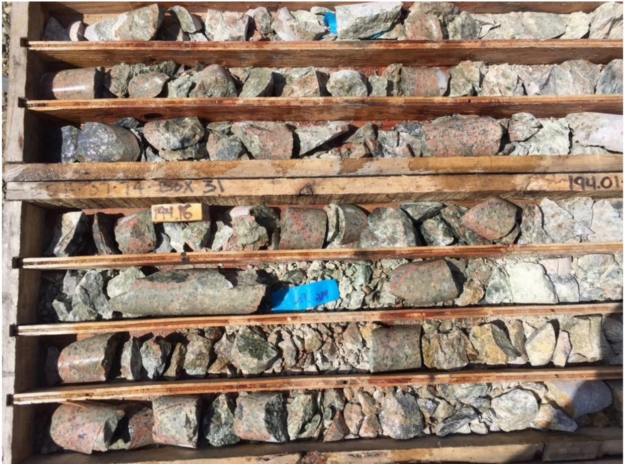
Figure 7-14: Mixed Potassic (k-feldspar) and Phyllic (sericite) Alteration, East zone, DDH 107, centered at 194.0 m (Lane, 2019)
