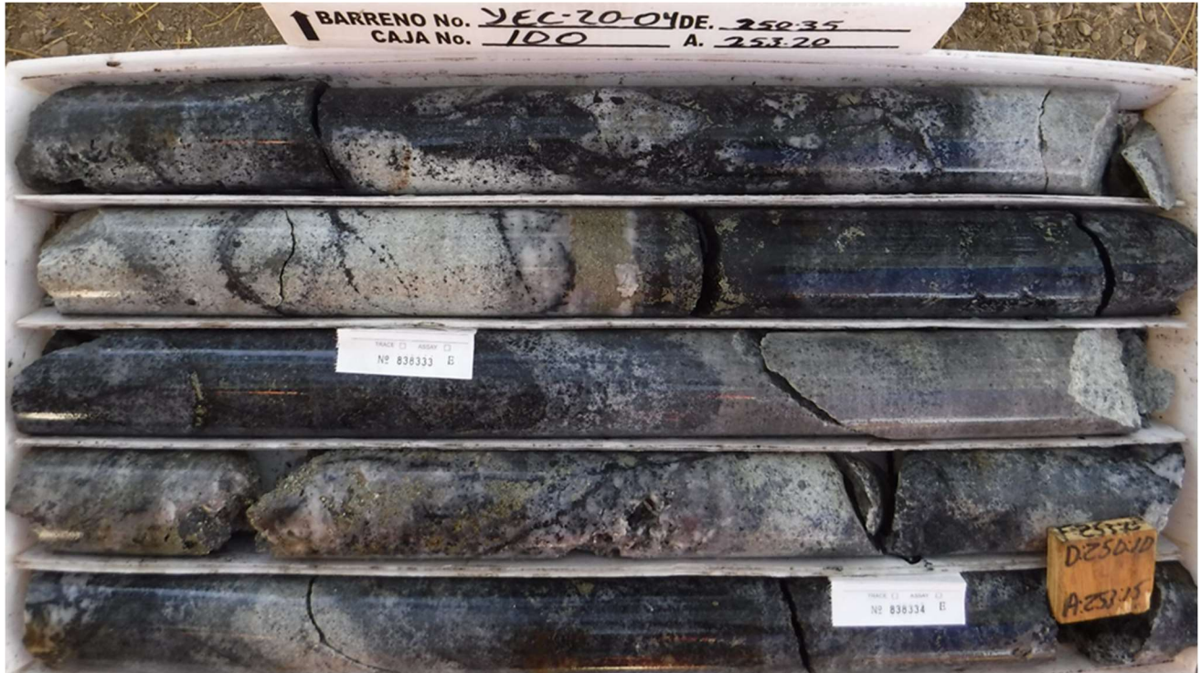
Figure 7.7 Core box of mineralized quartz tourmaline breccia from drill hole YEC-20-04 250.35-250.20 meter depth.
