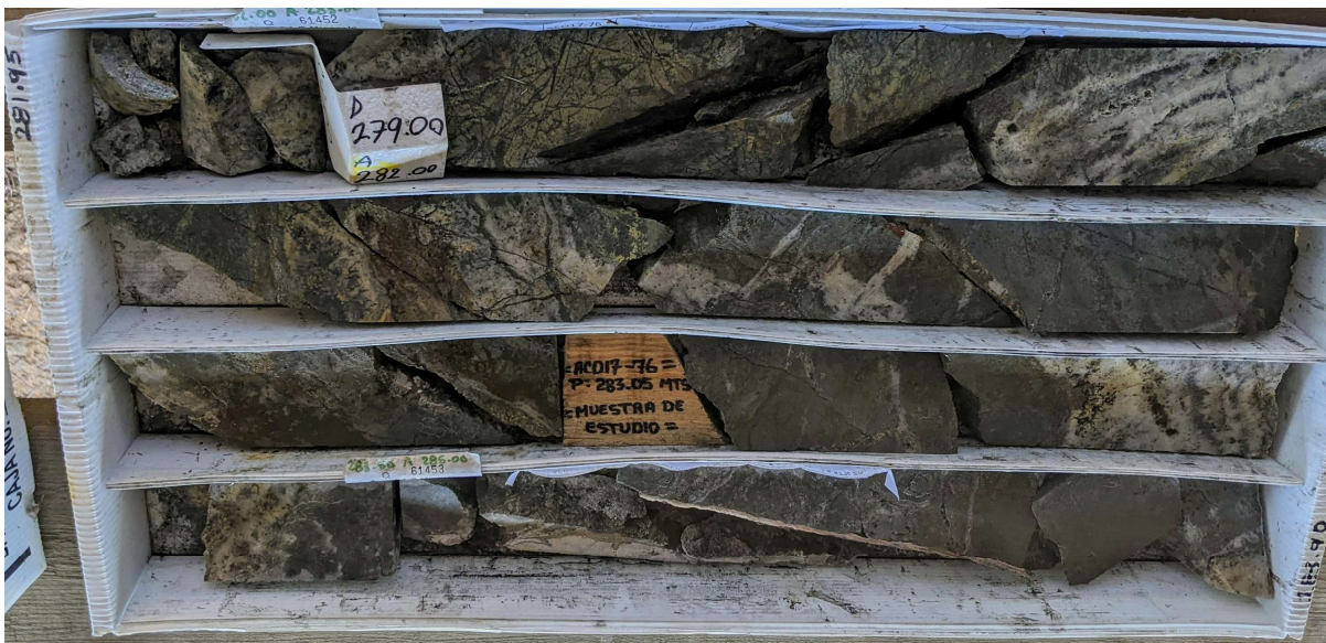
Figure 7.7: Mineralized Interval in Eastern End of Guadalupe Vein
