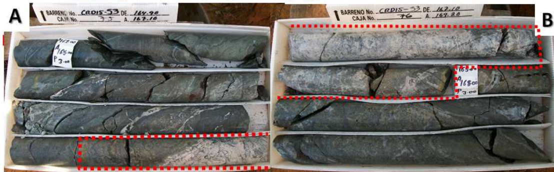
Figure 7.8: Adularia-rich Vein with Galena and Sphalerite on Margins
