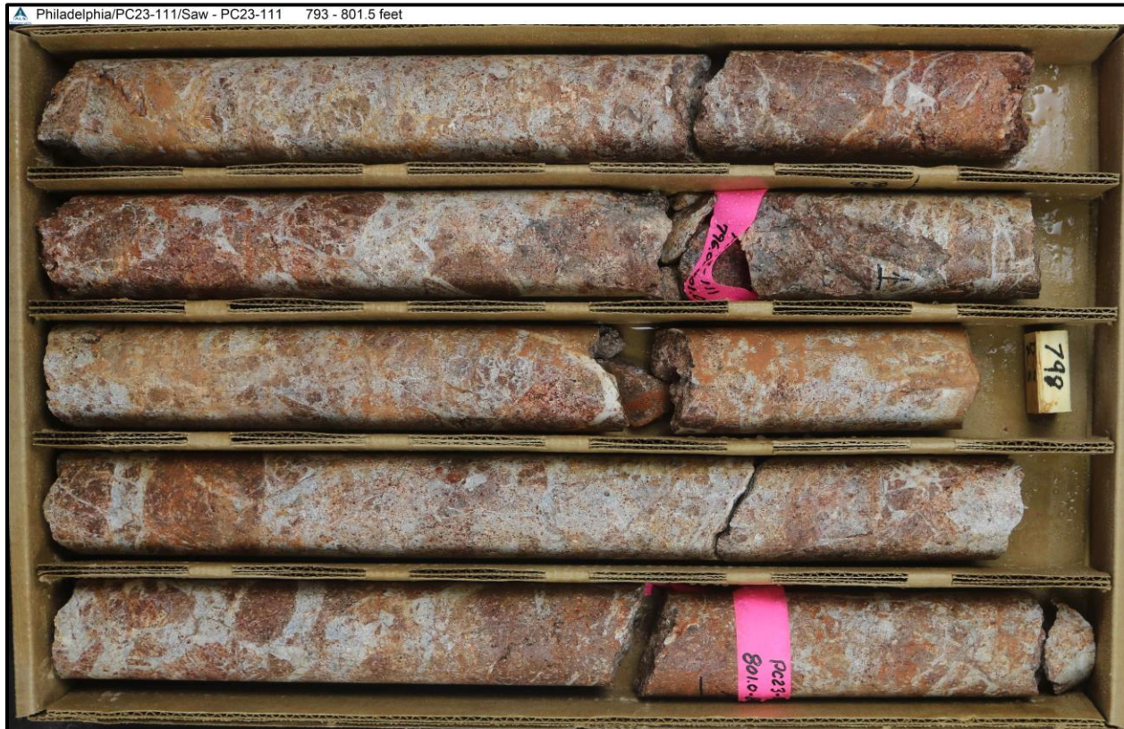
Figure 7.3-5 Tr2 rhyolite, dominant host to gold-silver stockwork mineralization.
