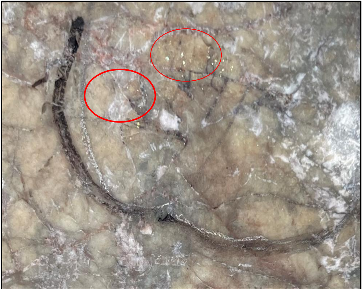
Figure 7.3-13 Fine-grained visible gold (in red circles) in drill core hole PC22-86.
