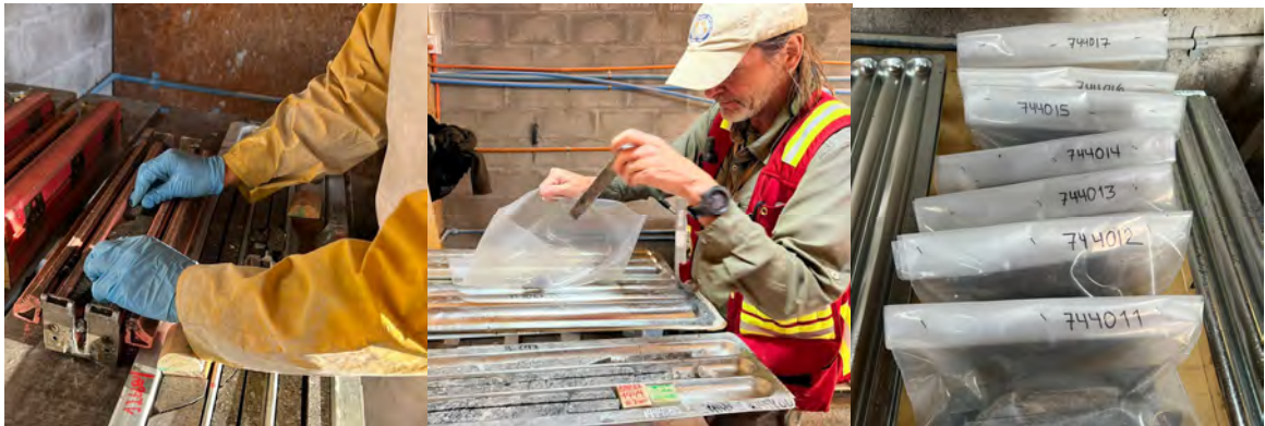
Figure 11-11: Left, preparation of \frac{1}{4} core by IMG sampler. Centre, bagging of \frac{1}{4} core samples by the QP. Right, sealed check samples ready for delivery to ALS laboratory in Santiago Chile.
