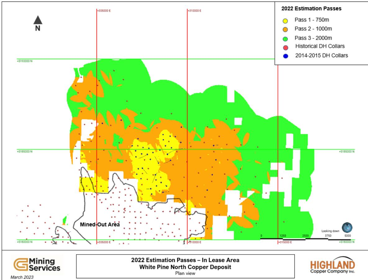
**Figure 14.15: Plan View of Pass 1 Search Ellipsoid (Parting Shale)**
