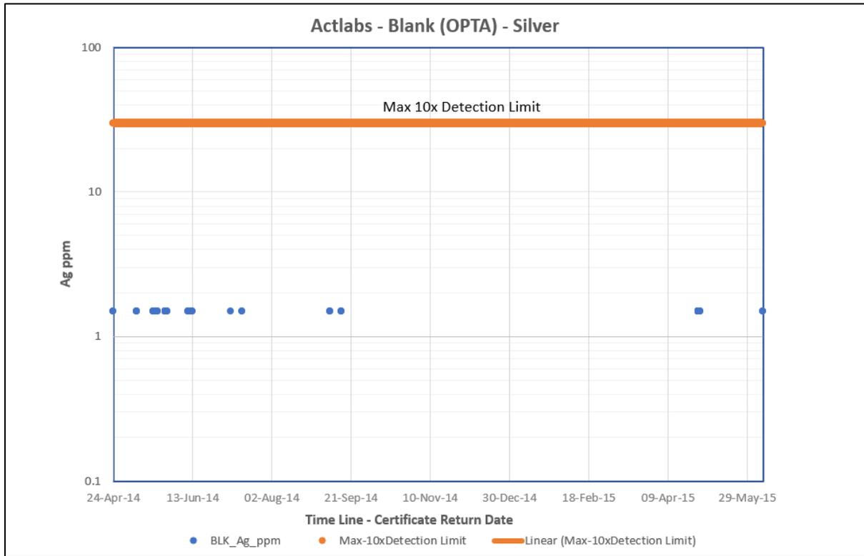
Figure 11.3 to Figure 11.6 show the analytical results for copper and silver observed by the BLK-10 certified blank material over time. In both charts, 100% of copper and silver blanks submitted were under the acceptable limits, and it is assumed that no significant contamination occurred during the sample preparation, delivery, and laboratory analysis.
