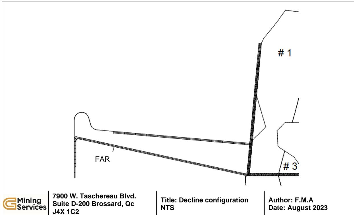
The mine consists of three mining sectors: West, Central and East. There is the main conveying system, and also strategically placed secondary conveying systems that are parallel to the panels. Each system is composed of four parallel drifts including: a fresh air intake drift, a mineralized material conveyor drift, a hauling drift, and a return air drift. Figure 16.4 shows the typical development drift configuration.
