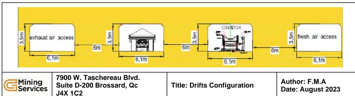
All drifts are set at a 6.1 m width, and their height varies from a minimum of 3.5 m to a maximum of 6.1 m. Most of the development will be performed by continuous miners. Continuous miners require a minimum opening of 3.5 m and can mine up to 5.8 m. Anything higher than 5.8 m would be mined with jumbos.
