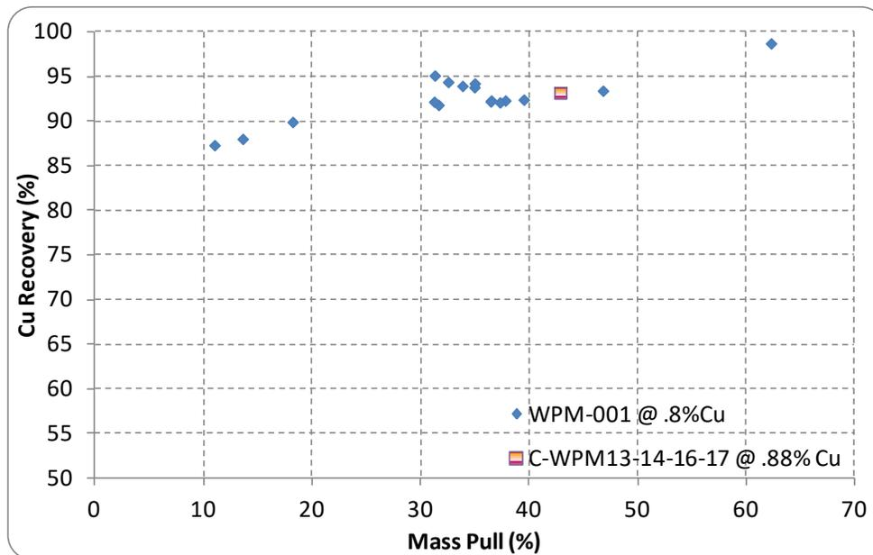
Subsequent open circuit flotation tests show that an FL2 flotation circuit could deliver interesting metallurgical performances. As indicated in Table 13.21 saleable concentrate grading up to 30% Cu could be obtained while recovering up to 90% of the copper in a LCT based projection. The selected reagent list was also very suitable for silver recovery indicating recoveries greater than 90%.
