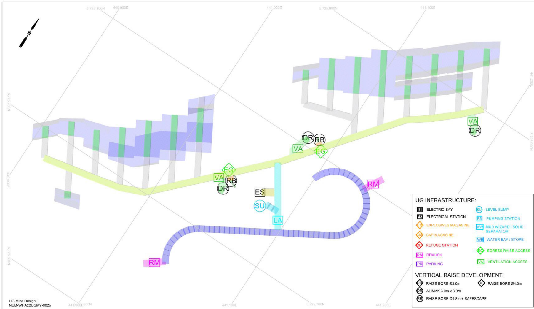
Figure 16-23 Typical 300L Layout
