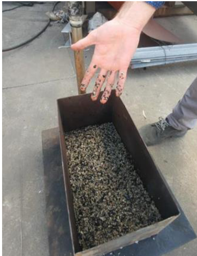
Figure 13-12 ThermoPower Drying Test #2, 80° Discharge Temperature
