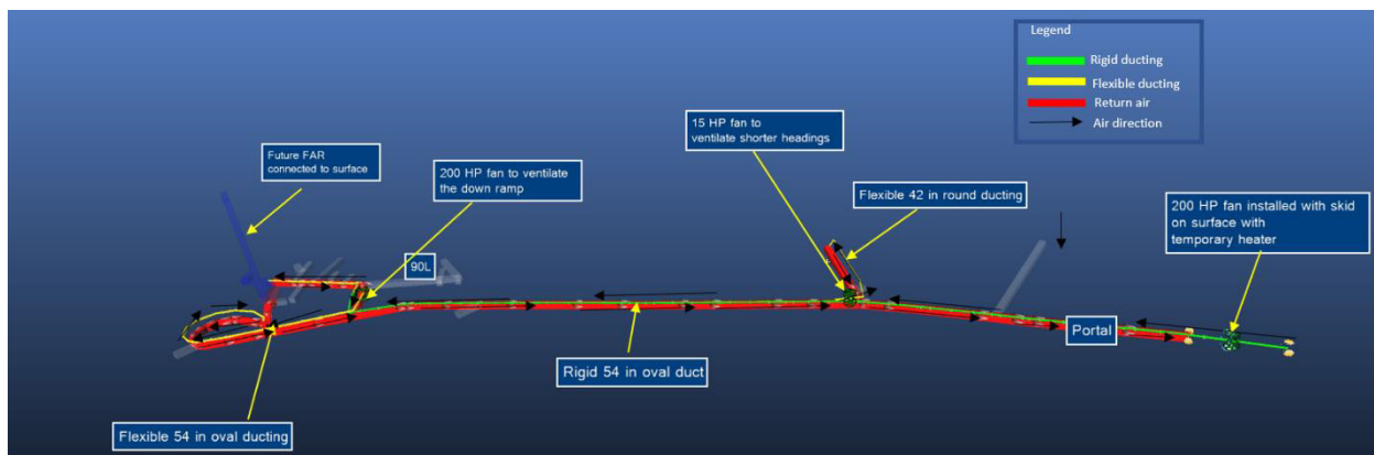
Figure 16-21 Ramp Development Ventilation Schematic
