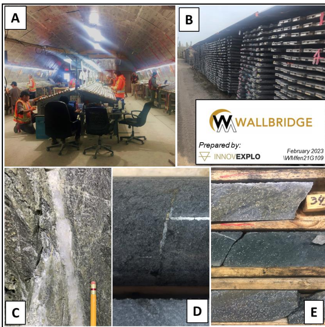
A: Core logging in action – B: Core yard – C: Underground exposure of the veins associated with the Interstellar 3 mineralized zone – D: Mineralized quartz veinlet in the mafic phase of the diorite of the Ripley (drill hole: FA-22-456 at a depth of around 196.0 m) – E: Sulphide-rich banding of the Martiniere West Trend (drill hole: MR-22-020 at a depth of 343.0 to 346.0 m)
