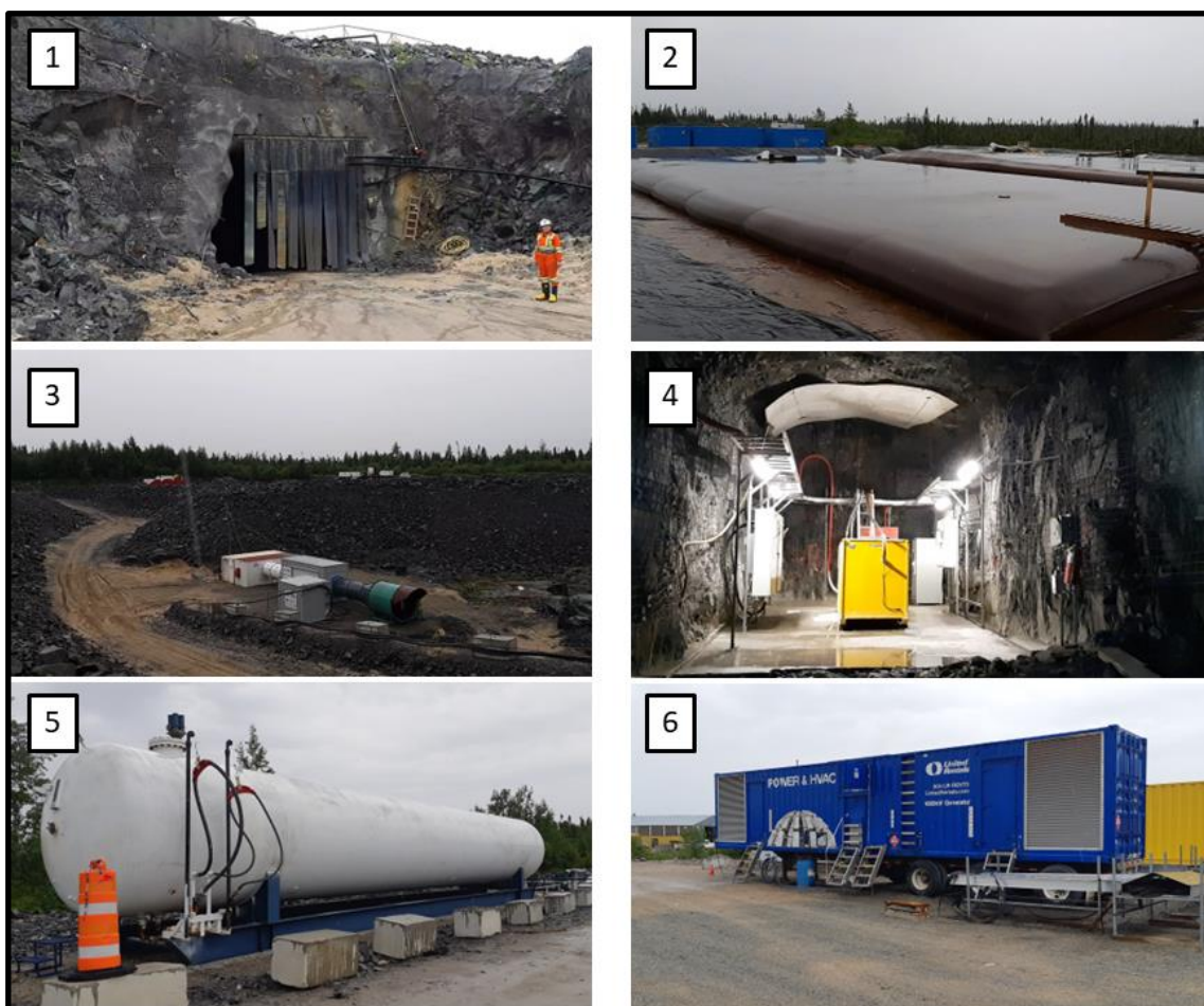
1: Portal entrance – 2: Geo-tube from the water treatment plant– 3: Underground ventilation and heater system – 4: Underground electrical sub-station – 5: Diesel fuel tank – 6: Mine site genset
