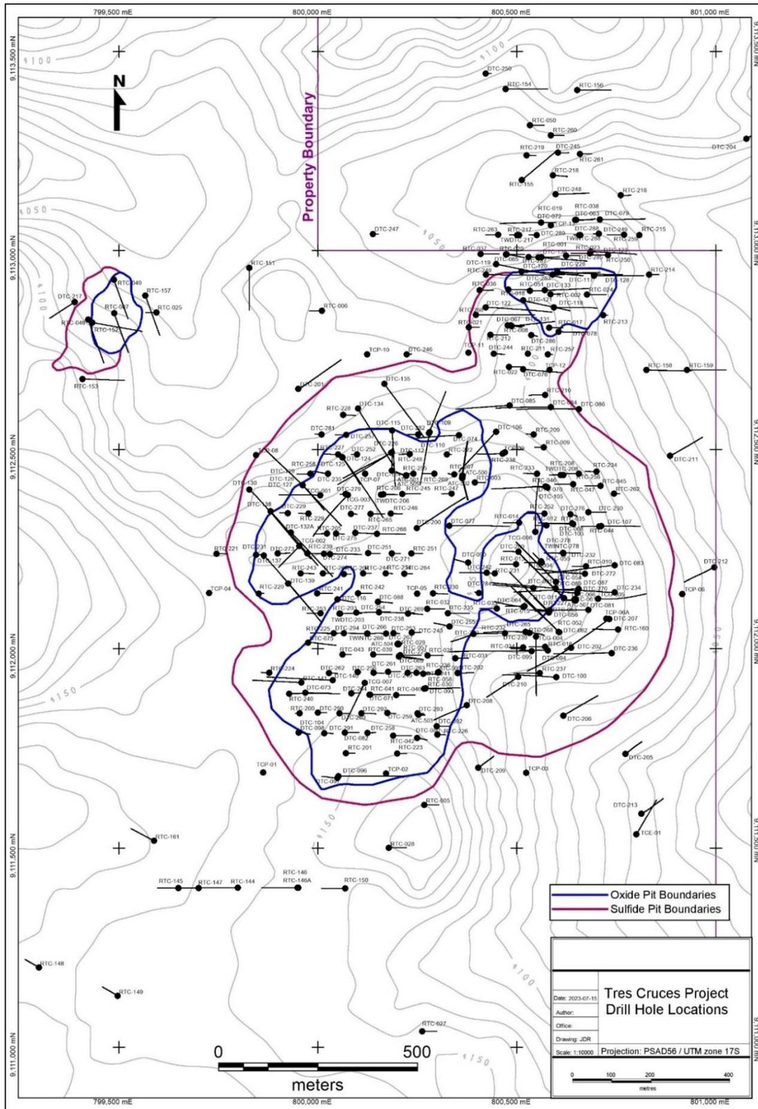
Figure 10-1: Drill Hole Locations and Proposed Pit Outlines
