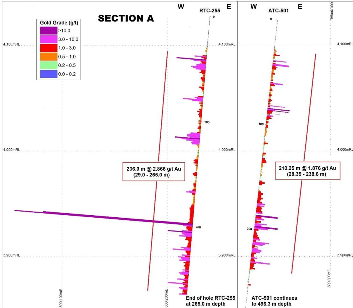
**Figure 10-9: Vertical Cross Section A, Viewed to the North**
