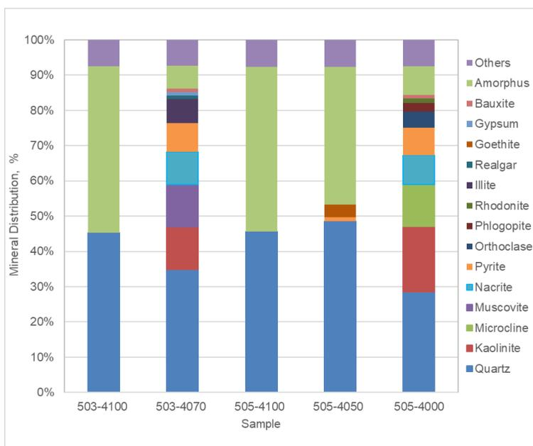
Figure 13-8: XRD analysis for samples
