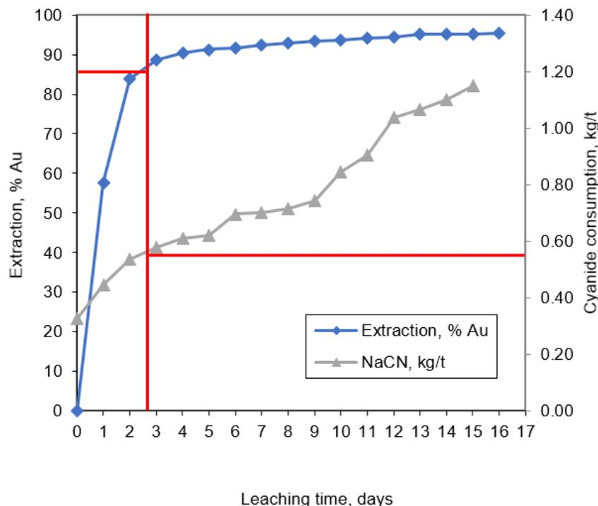
Figure 13-17: Example LC3, BMG short column gold extraction vs cyanide consumption, 1999.
