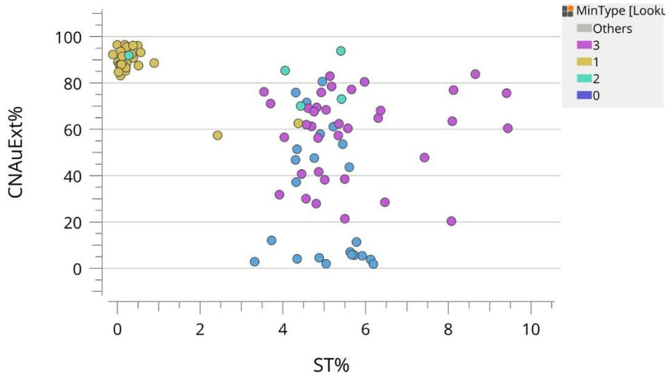
**Figure 13-14: Gold extraction dominated by direct cyanidation (CNAuExt%) by sulphur grade**
