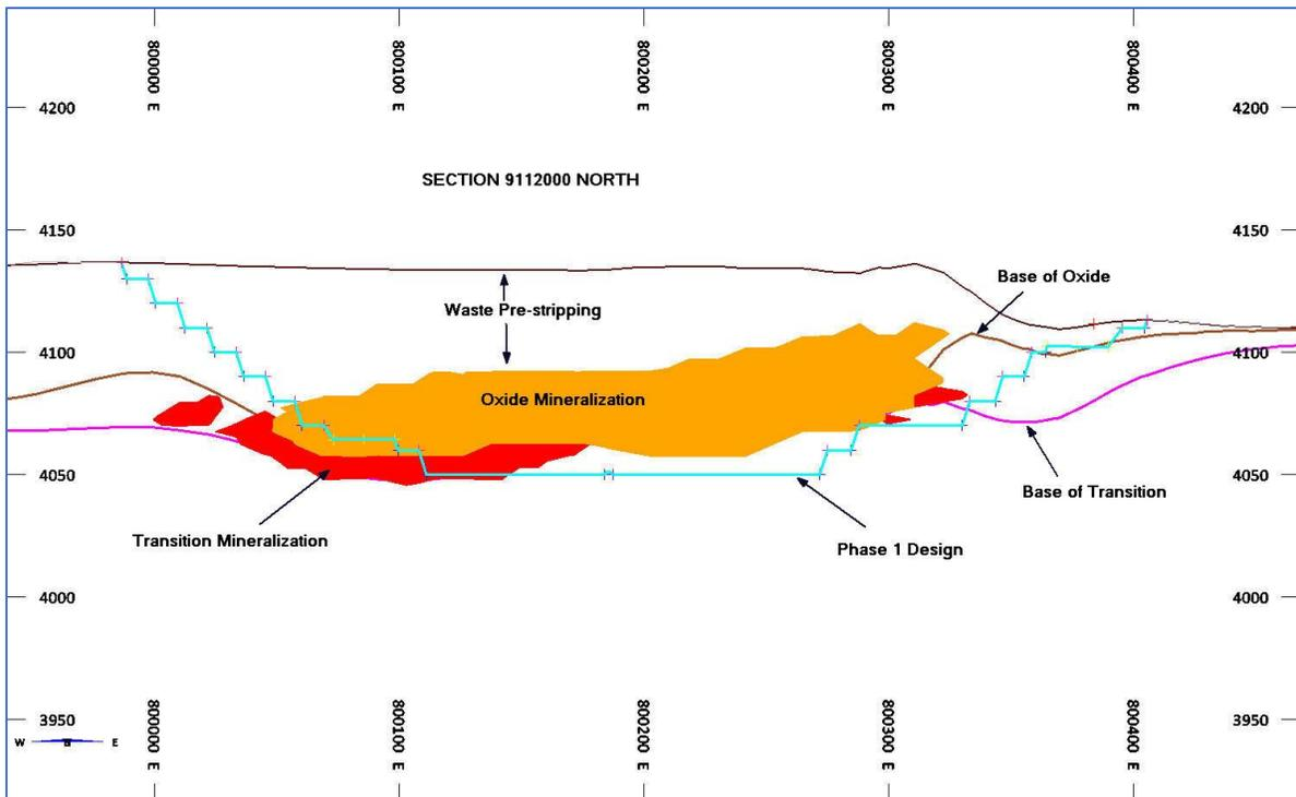
Figure 16-12: Phase 1 Design Section 9112000 North
