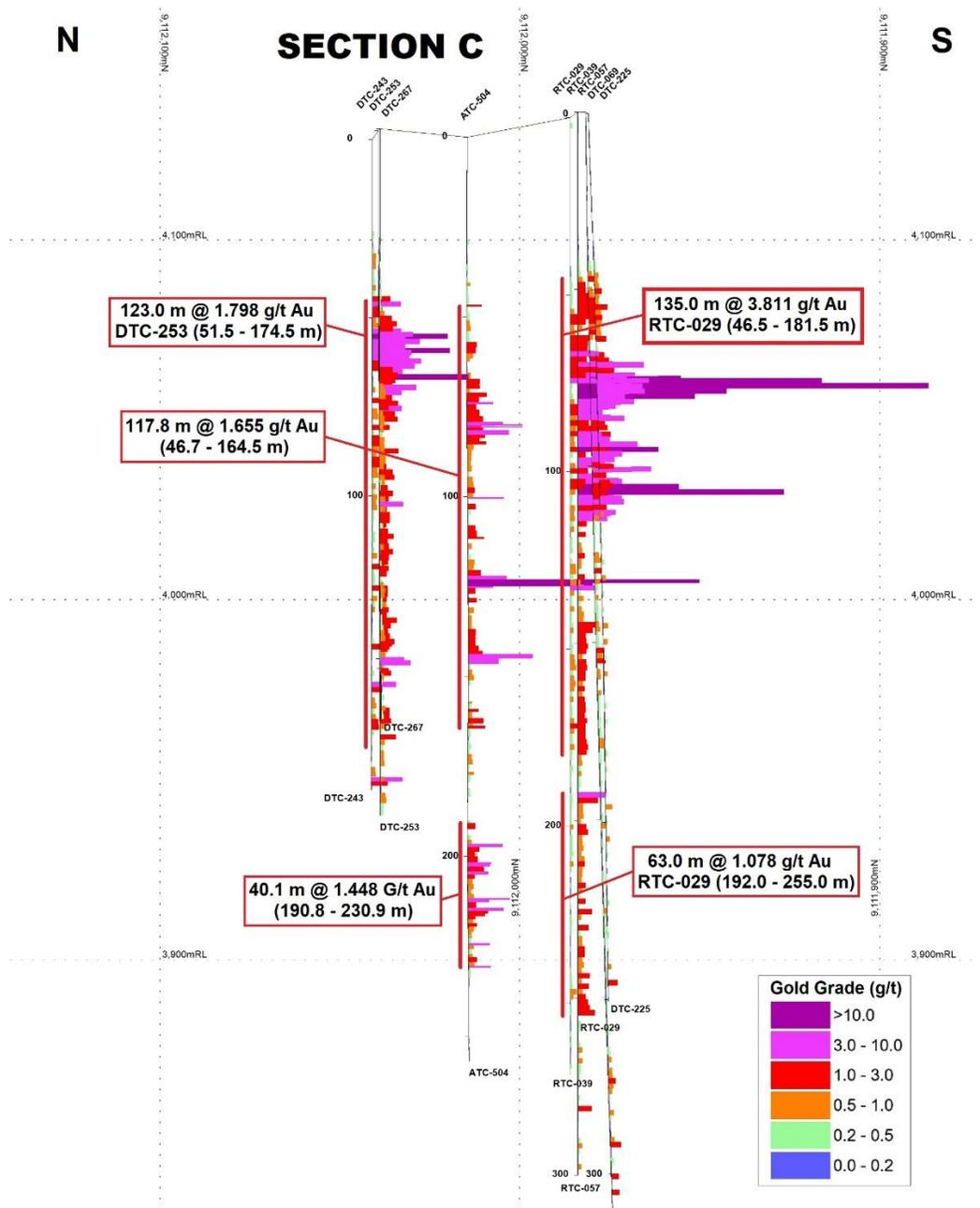
**Figure 10-11: Vertical Cross Section C, Viewed to the East**
