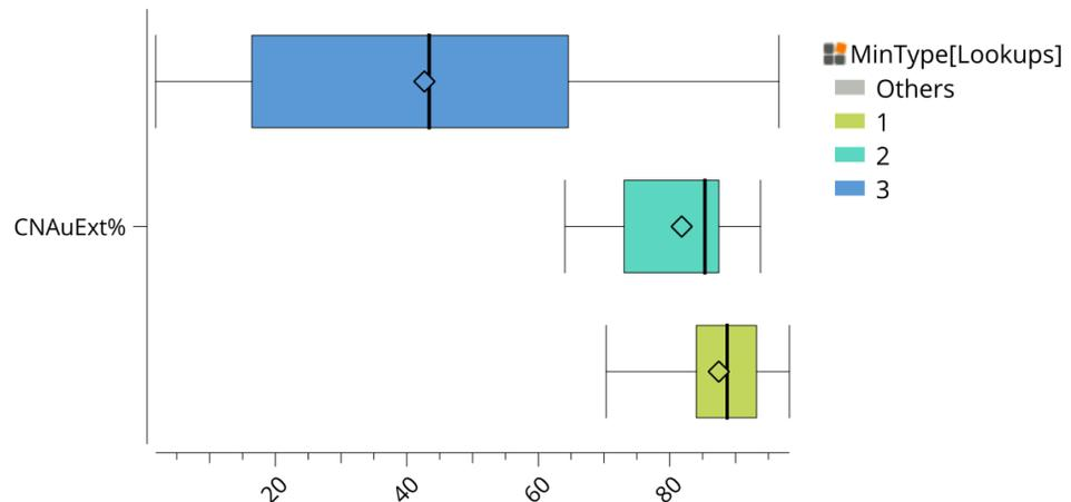
**Figure 13-15: Gold extraction by direct cyanidation (CNAuExt%) by MinType**
