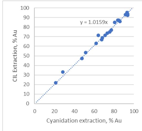
Figure 13-12: CIL extraction vs direct cyanidation extraction by AuTec
