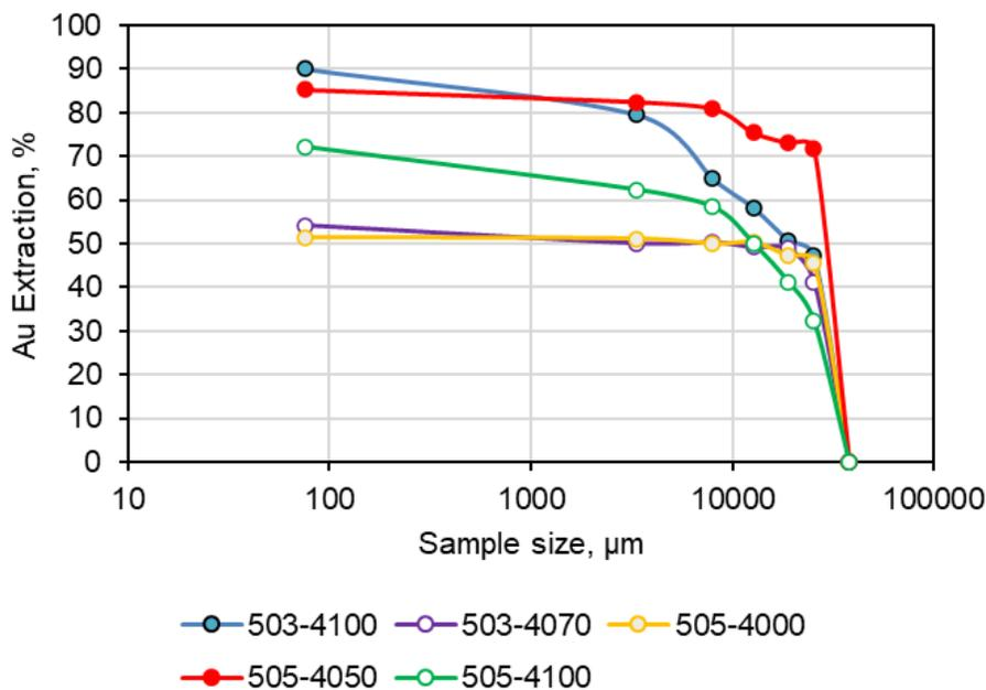
Figure 13-9: Cyanidation test for different particle size
