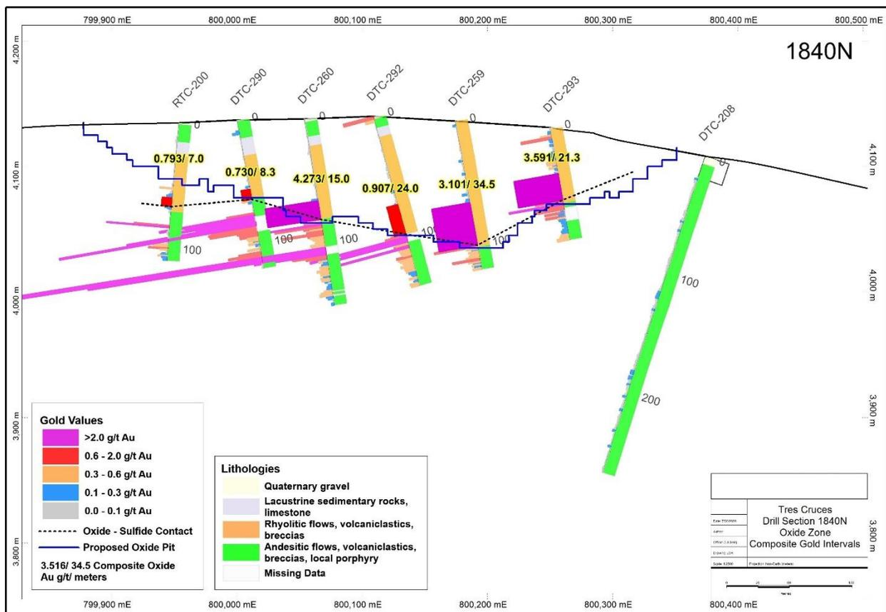
**Figure 10-3: Vertical Drill Section 1840N – Viewed at 360°**
