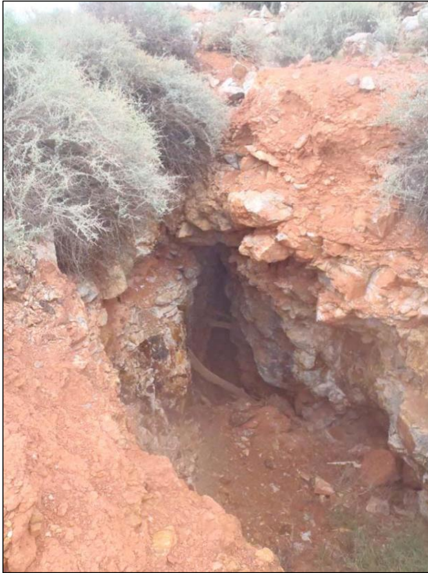
Figure 34 This photo was taken of the Weebo historical workings. The stope plunges to the east.
