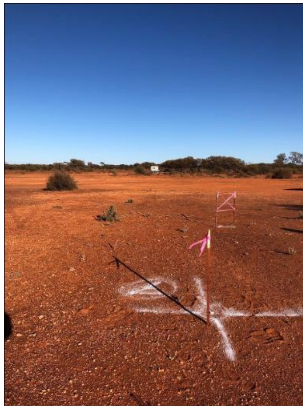
Figure 55 The temporary base station END2020 (in background) surveyed in from the Sir Samuel 47 base station.
