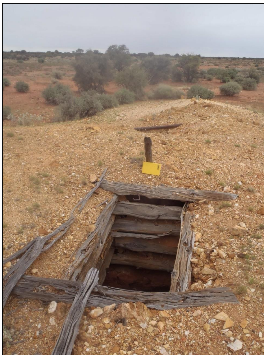
Figure 30 The mining shaft at Mermaid looking to the southwest. Note the second shaft beyond the notebook illustrating the sense of strike to the workings (striking 56°). This matches the 3D modelling of this mineralisation based on drill intercepts.
