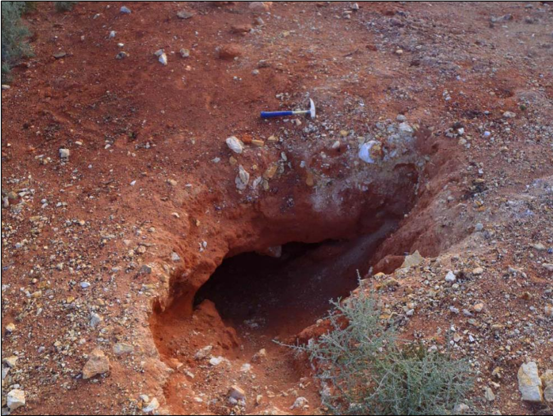
Figure 36 The historical stope of the Balmoral prospect. Visible in the hangingwall of the stope is the 10cm wide quartz vein that may have been the targeted structure.
