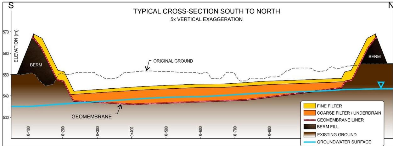
**Figure 18-7: TMF Pit North to South Cross Section**
