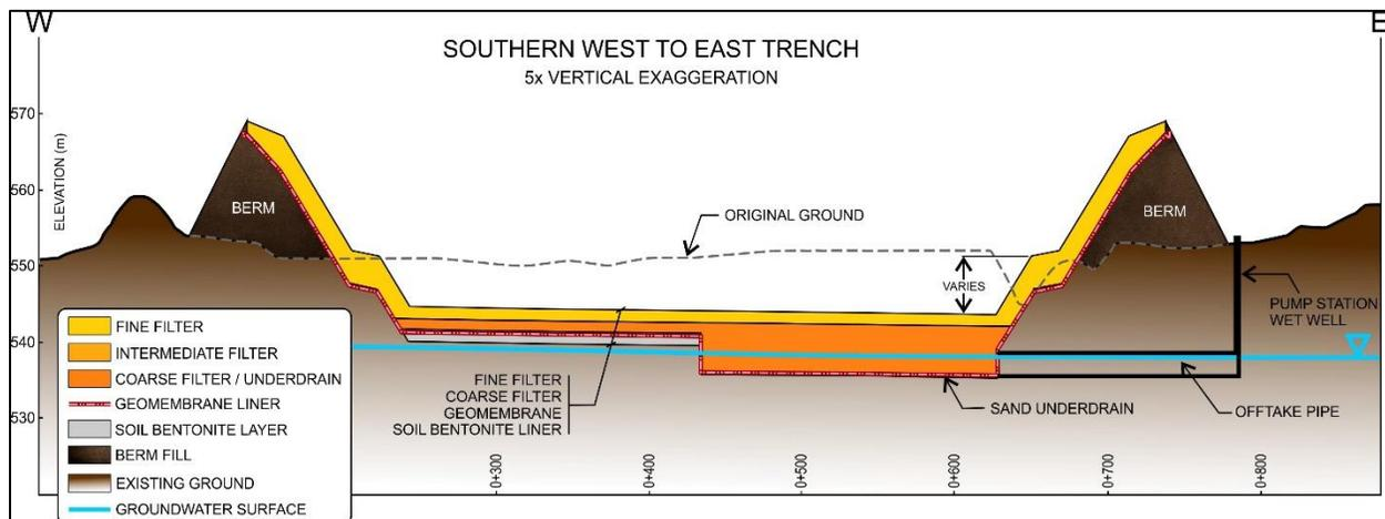
**Figure 18-6: TMF Pit East to West Cross Section**
