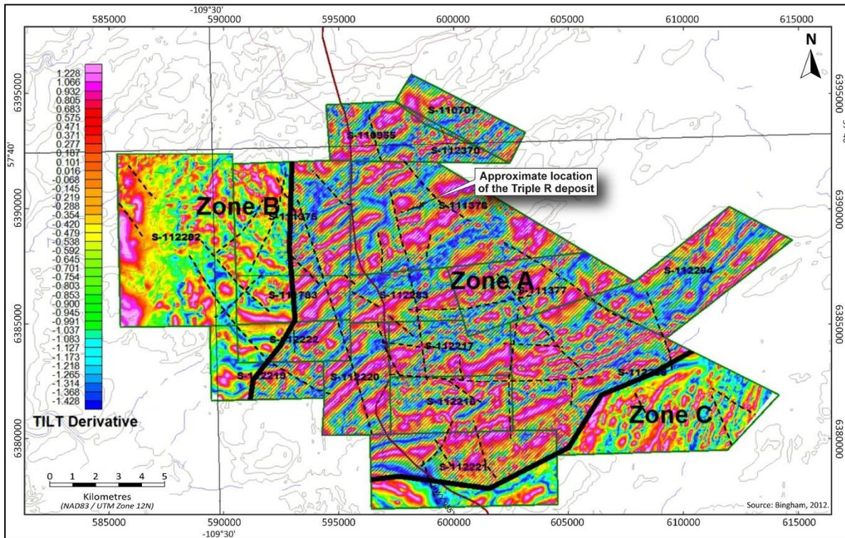
**Figure 9-2: Interpreted Major Structures and Tilt Derivative Magnetics**
