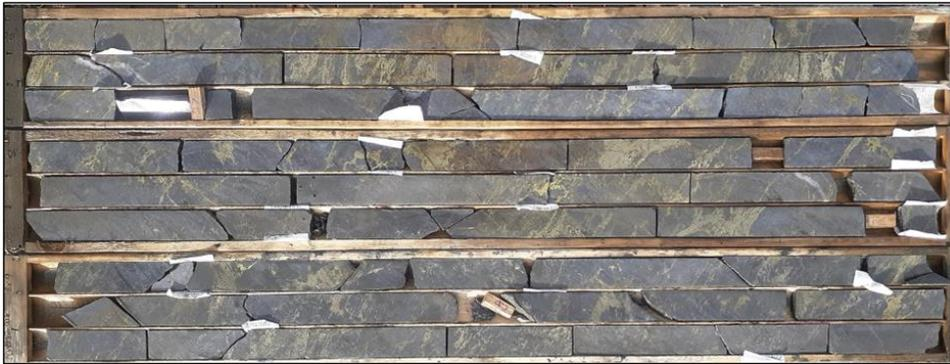
Figure 7.17: Mineralized interval, North Coldstream, Goldshore DDH CND-22-006
