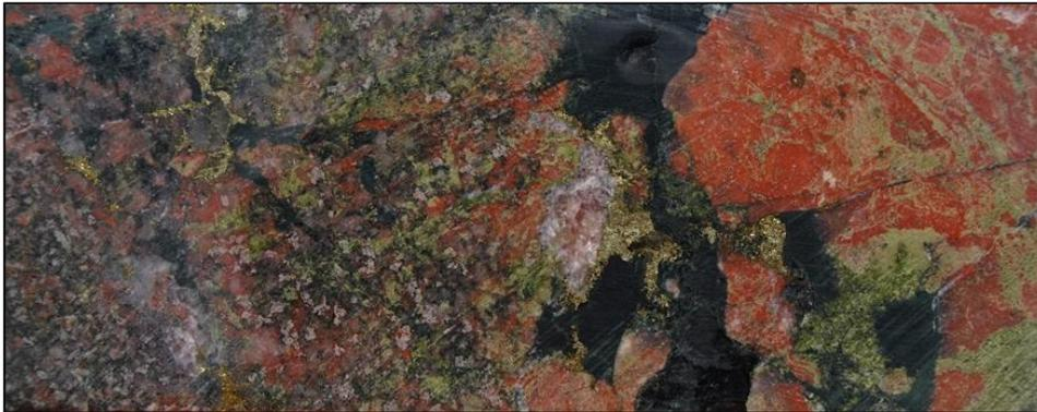
Figure 7.20: *Chalcopyrite-chalcopyrite mineralization at Hamlin in DDH HAM-11-75 as part of a chlorite-carbonate-epidote breccia overprinting hematite alteration*
