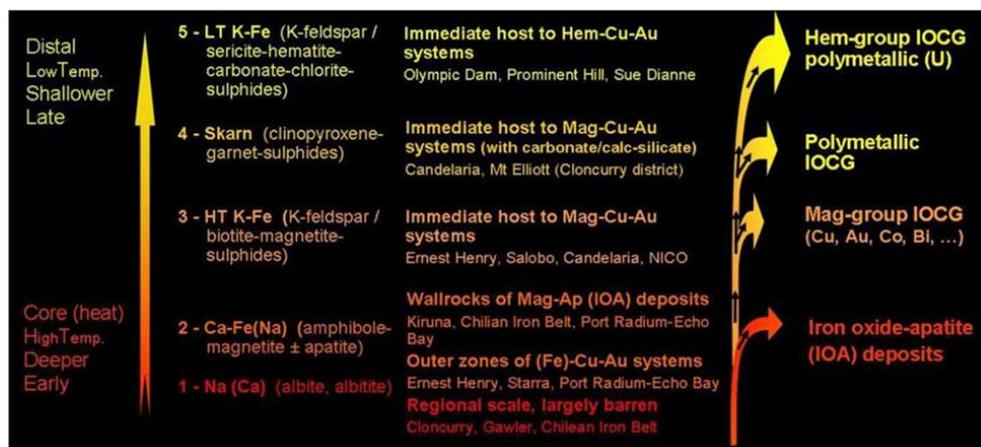
Figure 8.2: Progression of alteration in typical IOCG deposits (after Corriveau et al., 2010)
