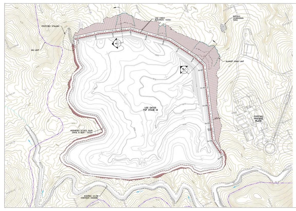
Figure 18.13: TSF Stage III Plan View (ultimate elevation)
