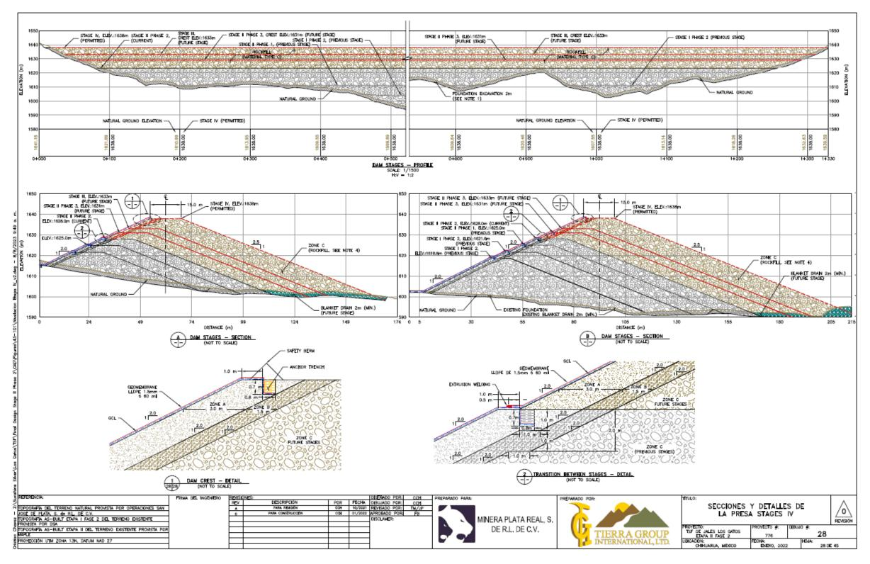
Figure 18.14: TSF As-Built and Future Stages Section View
