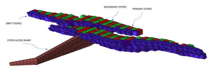
Figure 16.13: Schematic of Typical Transverse Cut-and-fill Stope Design at CLG
