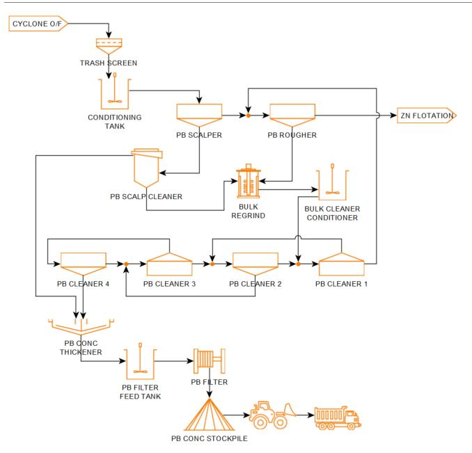
Figure 17.2: Lead Flotation Simplified Process Flowsheet
