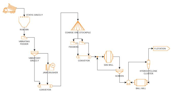
Figure 17.1: Crushing and Grinding Simplified Process Flowsheet
