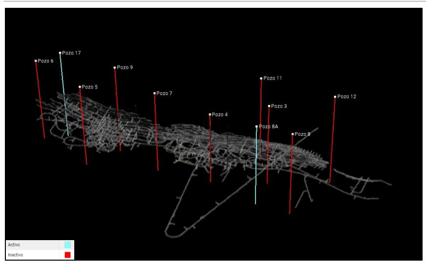
Figure 16.9: Isometric View Showing Surface Dewatering Wells and Mine Excavations
