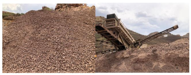
Figure 18.7: Astec KCI-JCI Mobile Jaw-cone Crushing Plant (left); -76mm Aggregate Stockpile (right)
