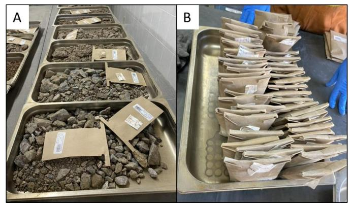
Figure 11.5: Left, Samples After Crushing I Right, Pulp Samples Labelled
