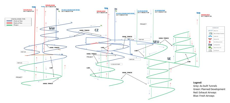
Figure 16.21: Heat Model Equipment Locations and Mine Heat Cooling Simulations Results
