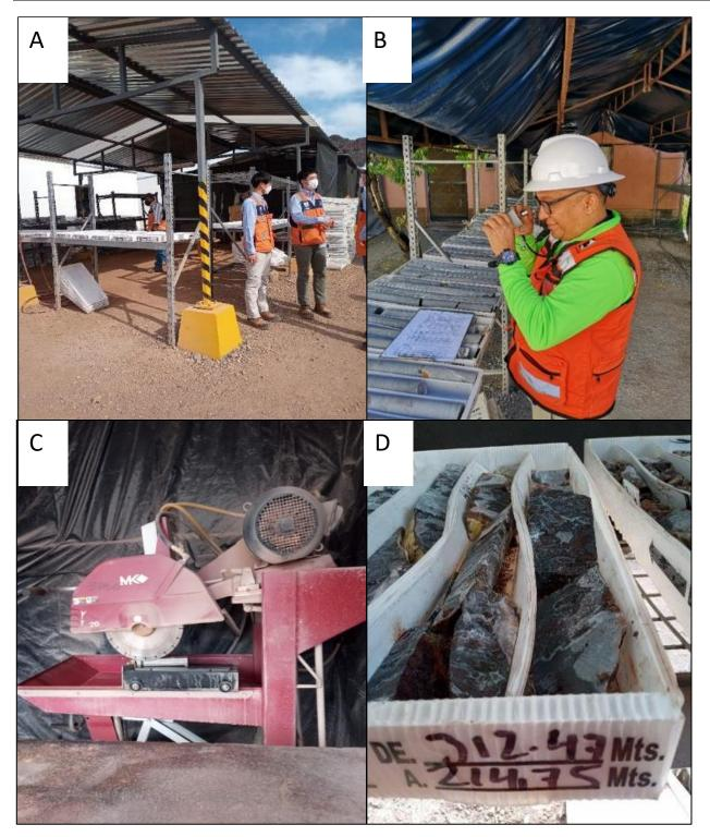
Figure 11.2: A) Geological Core-Shack; B), Geological Logging on Site; C), Electrical Diamond Saw; D), Half Core Placed in a Labelled Core Box
