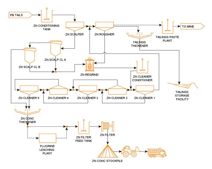
Figure 17.3: Zinc Flotation and Tailings Simplified Process Flowsheet
