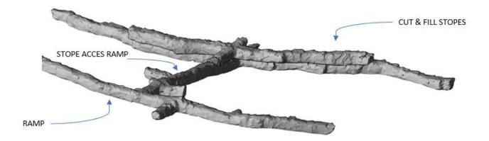
Figure 16.12: As-built Isometric View of Mining Longitudinal Cut-and-Fill Stopes at CLG
