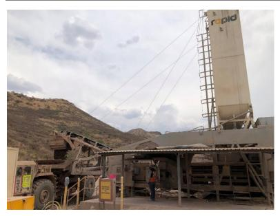
Figure 18.6: CRF Production at the Rapid Mix 400C Plant
