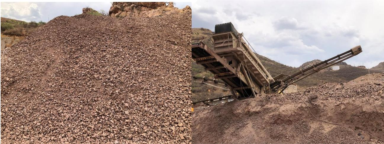
**Figure 18.7: Astec KCI-JCI Mobile Jaw-cone Crushing Plant (left); -76mm Aggregate Stockpile (right)**
