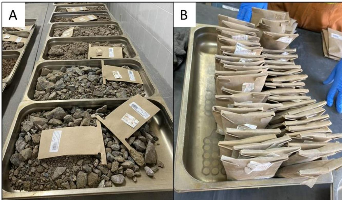
Figure 11.5: Left, Samples After Crushing | Right, Pulp Samples Labelled
