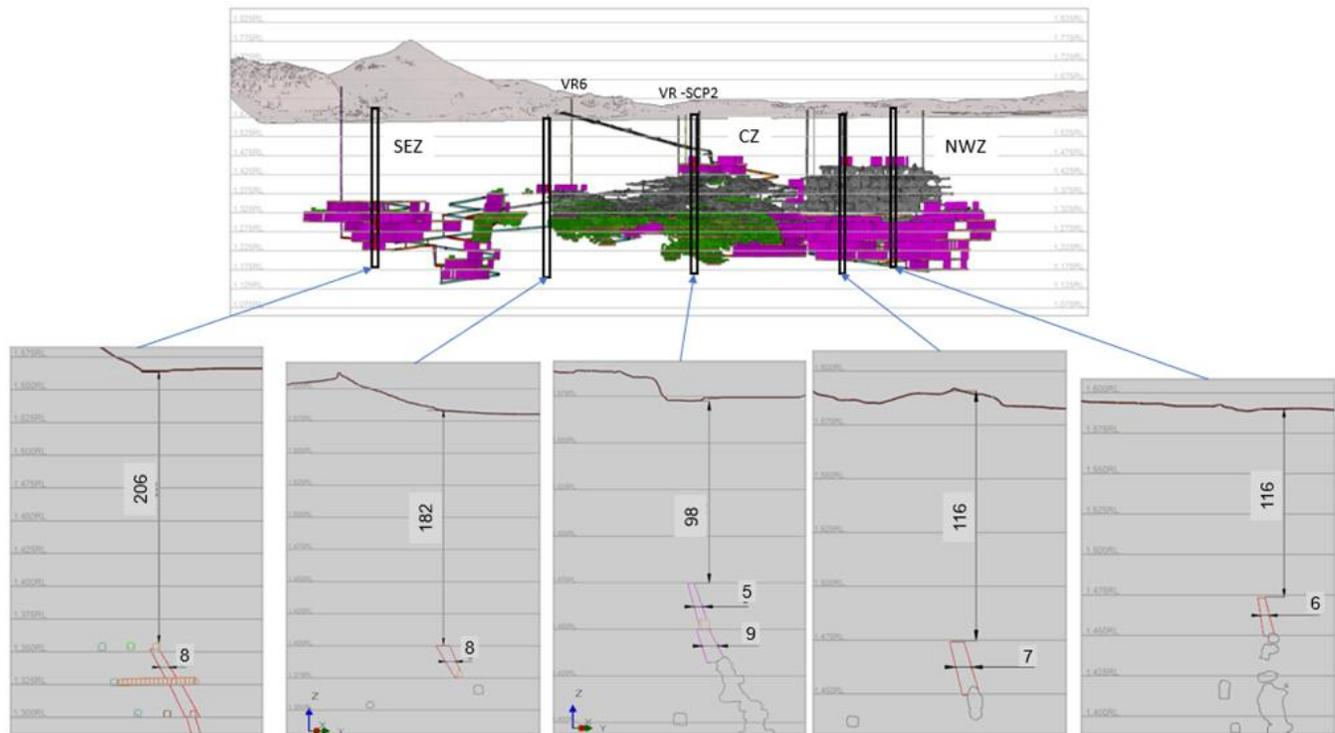
**Figure 16.7: Crown Pillar Thickness Along Deposit Strike**
