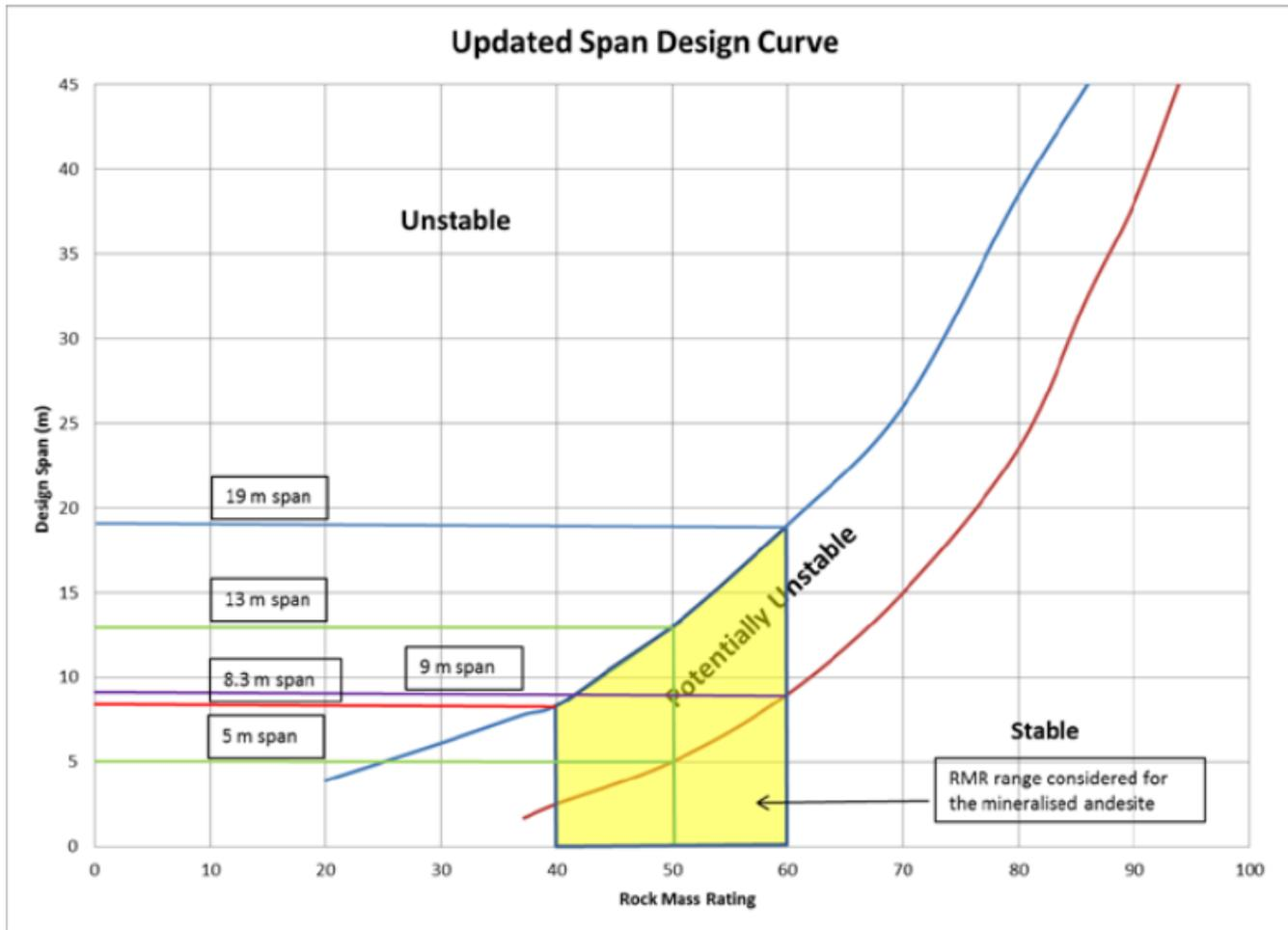
**Figure 16.5: Design Span for CLG Cut-and-Fill Stopes**
