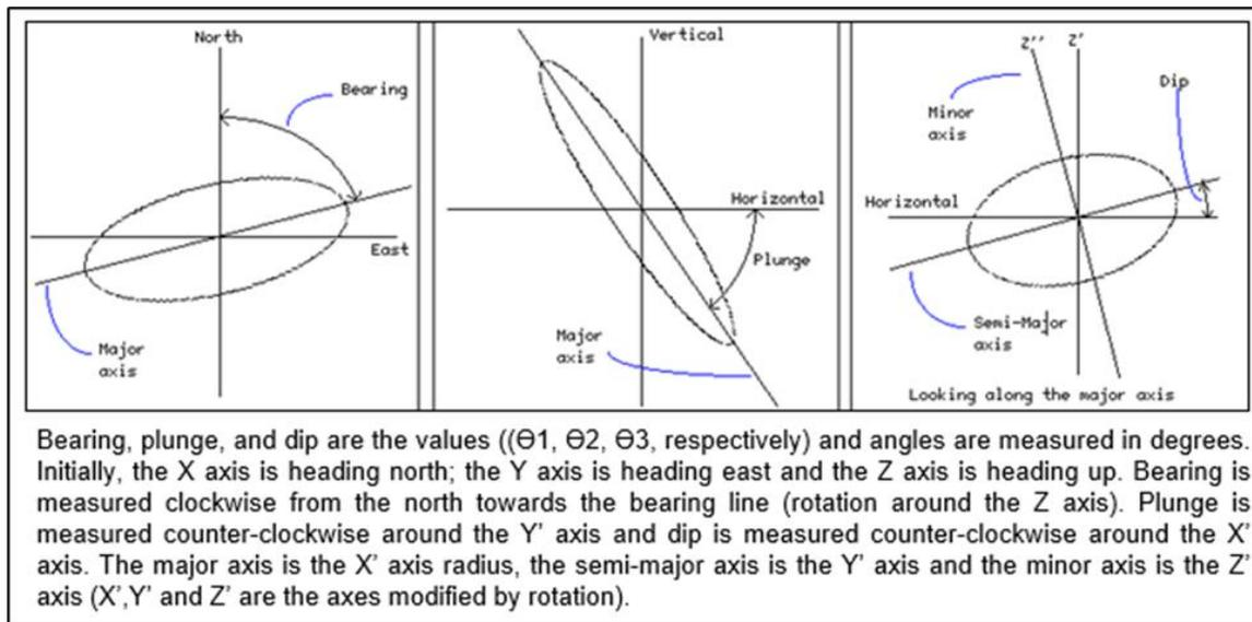
**Figure 14.8: Angle and Axis Convention in Vulcan**
