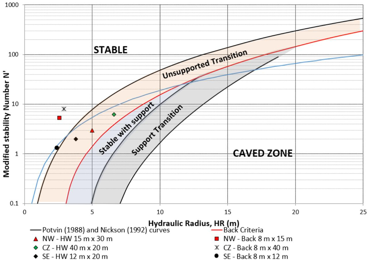
**Figure 16.6: Stability Graph for Transverse and Longitudinal Stopes**
