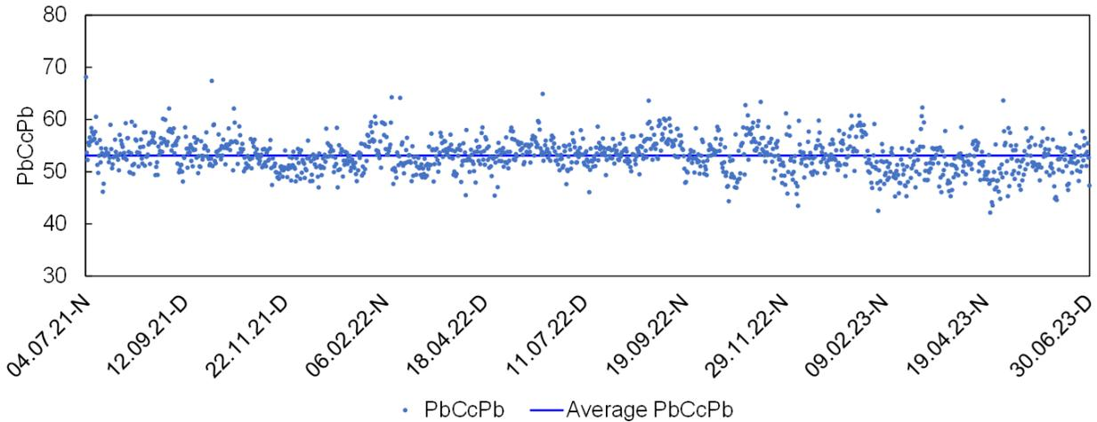
**Figure 13.20: Time Plot of Plant Lead Concentrate Grade**
