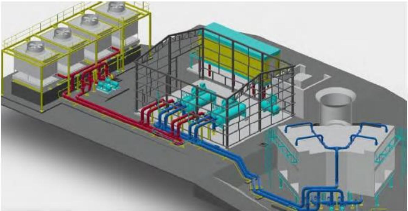
Figure 18.2: 3D Rendering of Refrigeration Plant 2 Design
