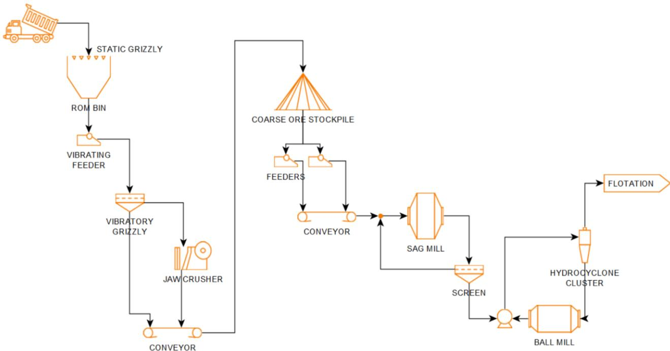
Figure 17.1: Crushing and Grinding Simplified Process Flowsheet
