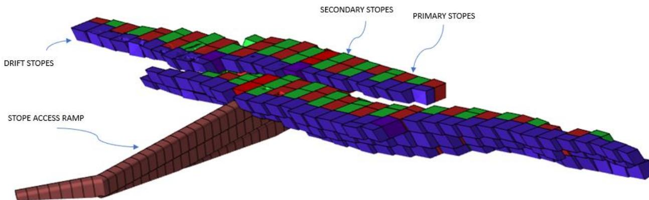
Figure 16.13: Schematic of Typical Transverse Cut-and-fill Stope Design at CLG
