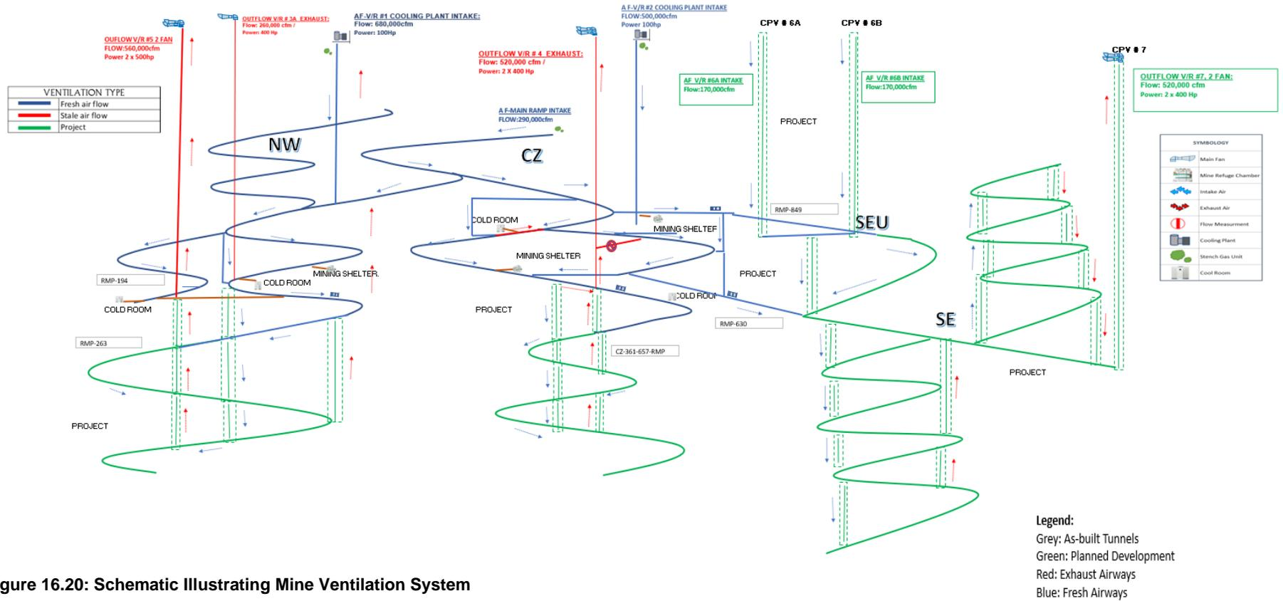
Figure 16.20: Schematic Illustrating Mine Ventilation System
