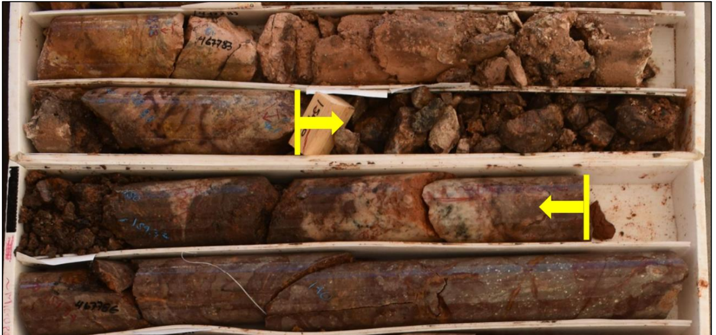
Figure 7-26: Drill Hole BAS22-209, from 159.00 to 160.45 m at 1.0 m (True Thickness) Grading 38.12 gpt Au and 165.0 gpt Ag
