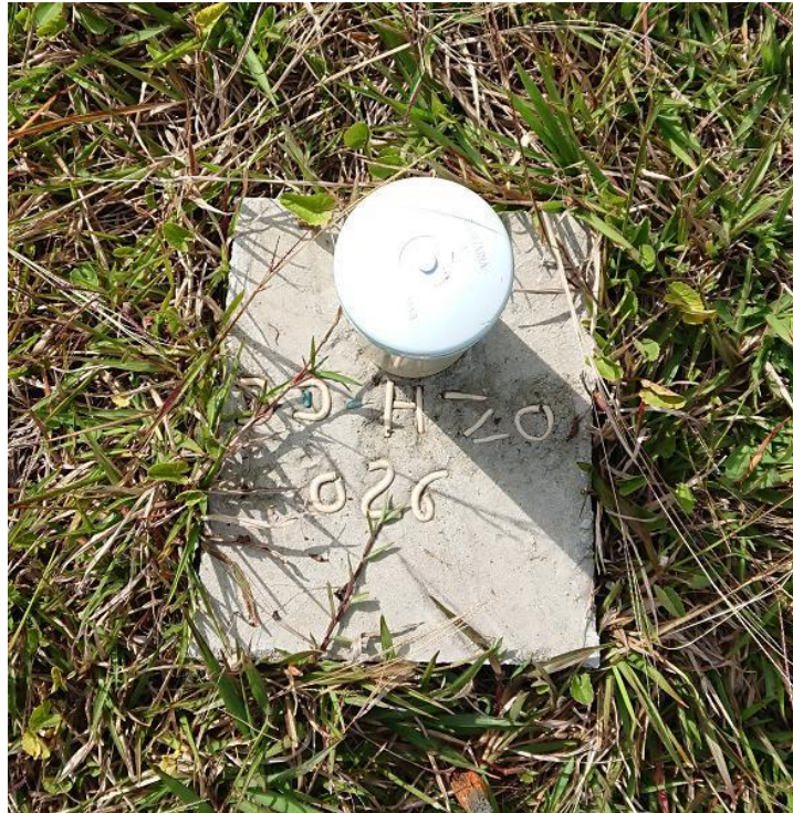
Figure 10-2: Collar Monument of DDH-ZO-026 at La Cumbre Area
