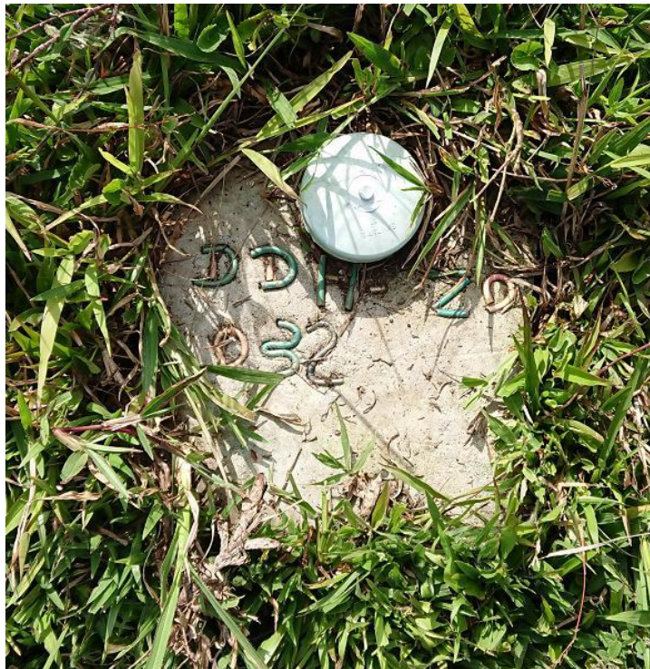
Figure 10-4: Collar Monument of DDH-ZO-032 at La Cumbre Area
