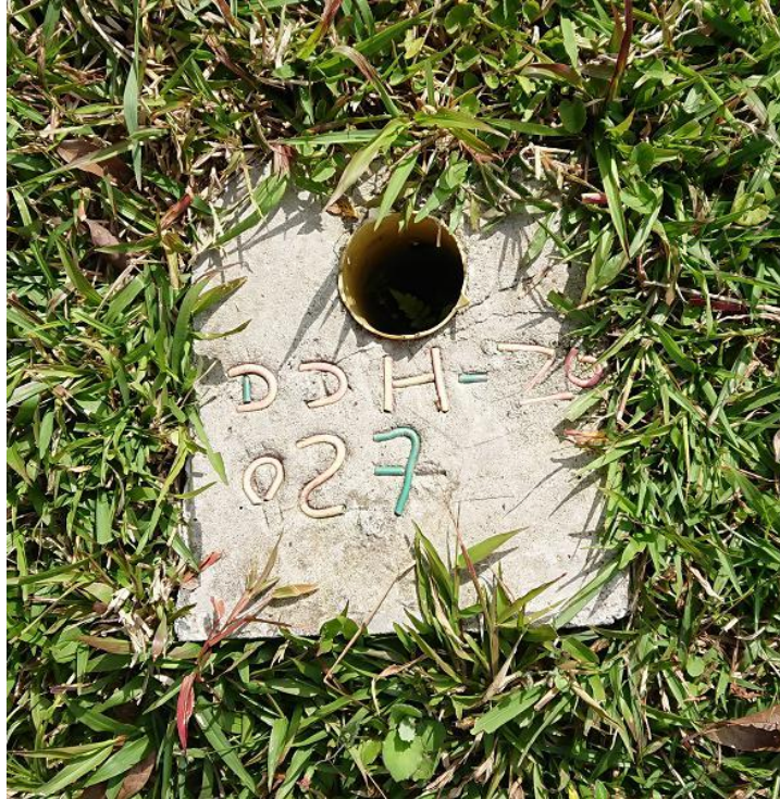
Figure 10-3: Collar Monument of DDH-ZO-027 at La Cumbre Area
