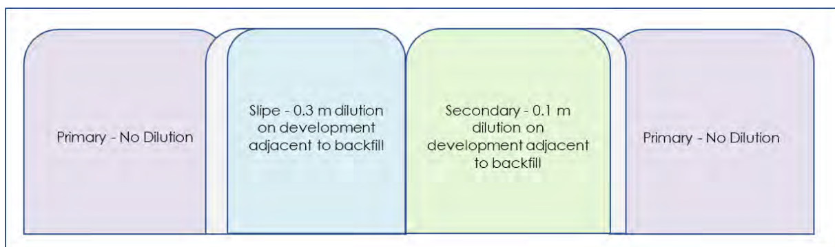
Figure 16.34 Typical Drift-and-Fill dilution due to overbreak into backfill
