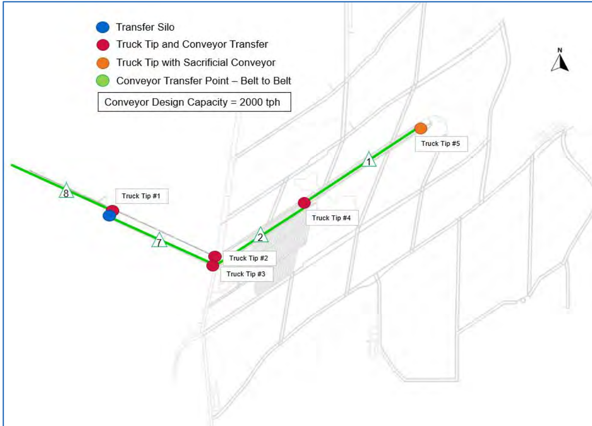
Figure 16.70 Kamoa 1 Mine Underground Rock Handling Conveyor Routing
