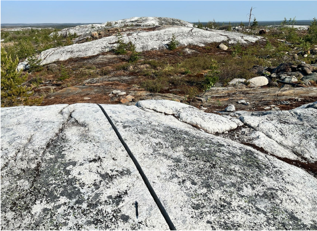
Figure 12-2 – Channel Sample Across Pegmatite Outcrop
