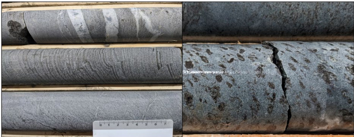
Figure 7-4 – (Left) Typical paragneiss textures with preserved bedding. (Right) Biotite-rich porphyroblasts in mafic intrusive
