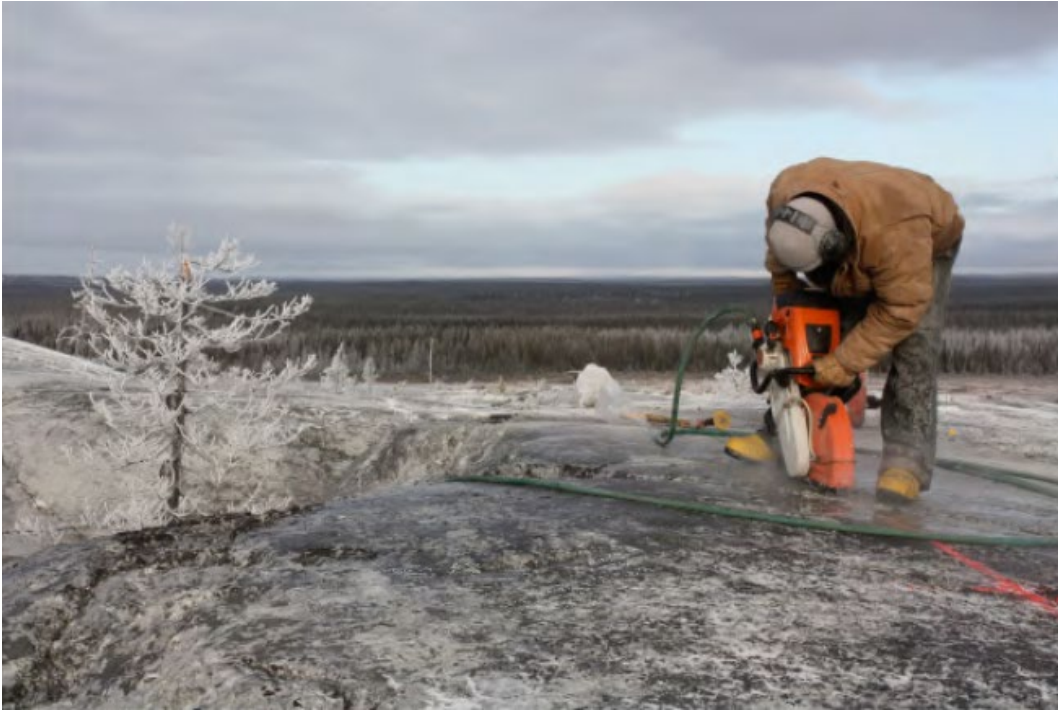
Figure 10-3 – Channel Sampling in 2011 Using a Double-Bladed Circular Saw
