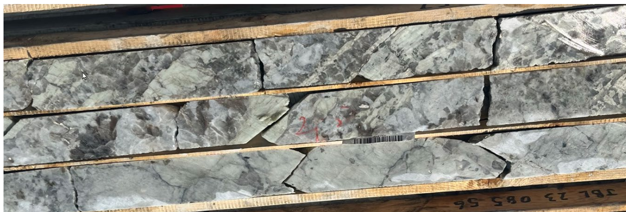
Figure 12-1 – Abundant Light Green, Coarse-Grained Spodumene in JBL-23-85
