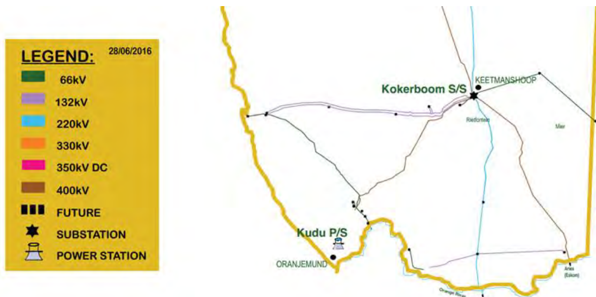
Figure 16-3: Power Line Transmission and Substations in the South of Namibia.
