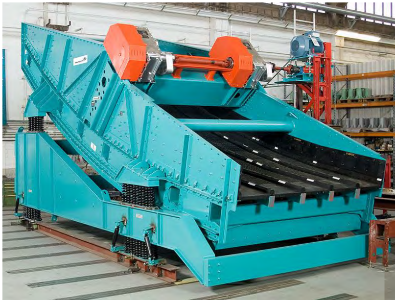
Figure 14-3: Typical secondary screen
