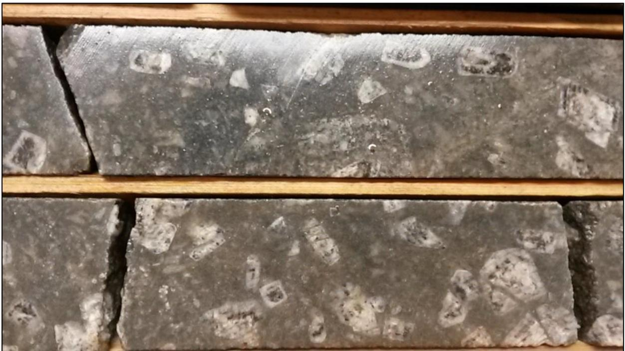
**Figure 7-5 Porphyry with large Phenocrysts of Feldspars**
