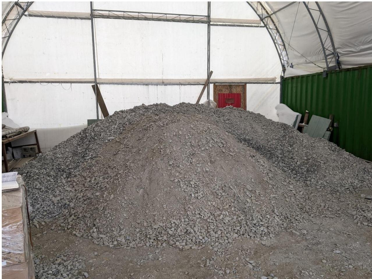
**Figure 12-4 Bulk Material Stored in a Shelter**
