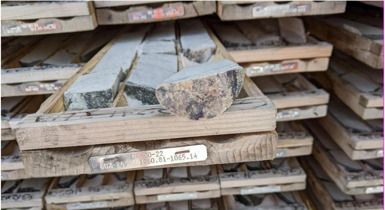
**Figure 12-10 GR-20-22 from 1060 to 1065 m with Purple Mineral as Fracture Filling**
