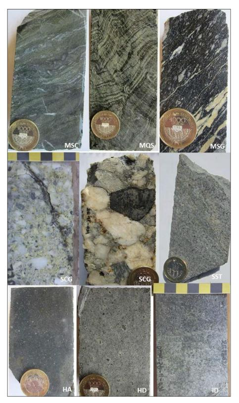
Notes: Top row: MSC, Chlorite schist; MQS, Quartz sericite schist; MSG Graphite schist. Middle row: SCG Conglomerate, SST Sandstone. Bottom row: HA, Andesite porphyry; HD, Dacite porphyry; ID, Diorite. Source: IAMGOLD, 2020 and photos by S. Redwood.
