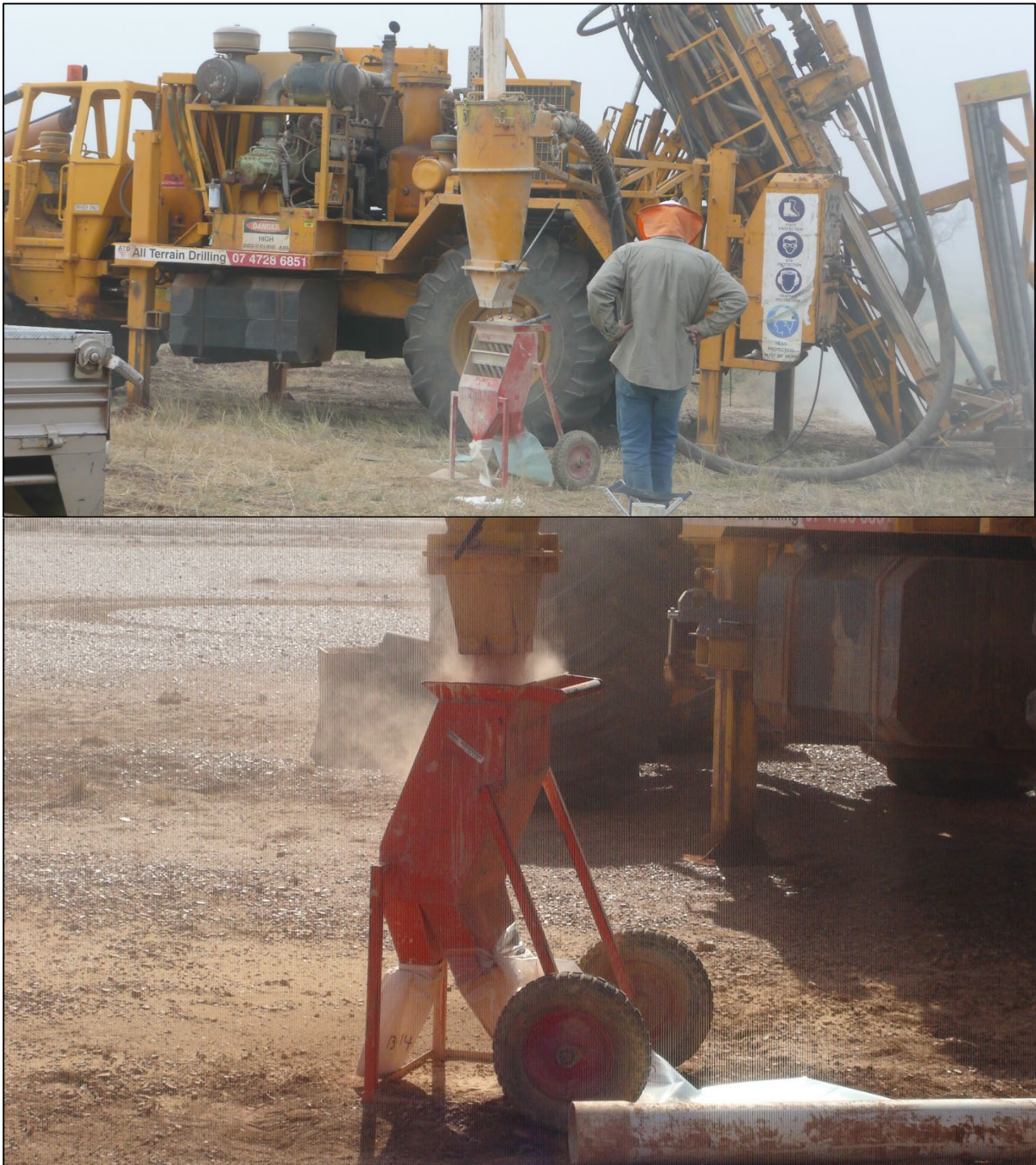
Figure 11-1. Photographs of RC drill rig, cyclone, and riffle splitter configuration.
